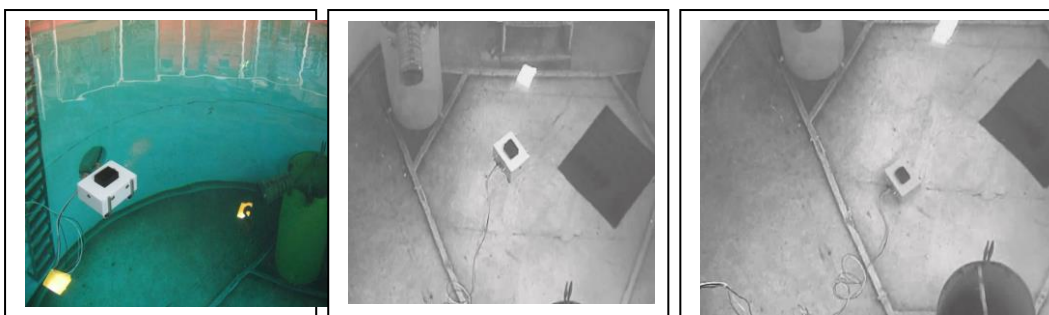
Figure 14: The FPSO robot swims to a test location and descends (using active buoyancy control) to the floor. It uses wheeled motion on the floor to move along strengthening plates and perform weld inspection
