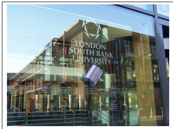
Figure17: VORTEX climbing on glass surface
