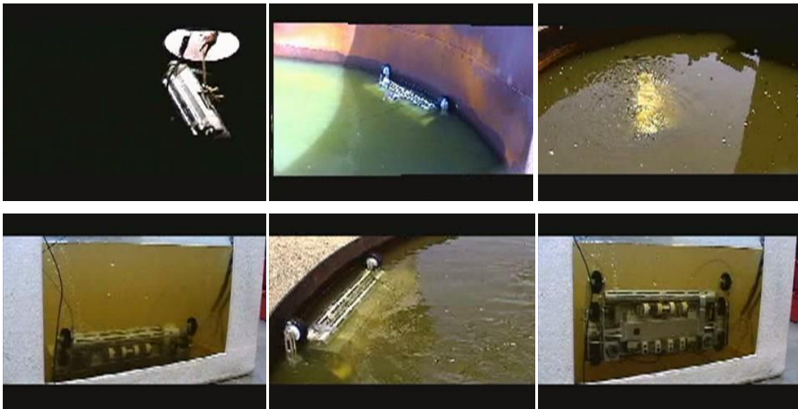
Figure 4. RobTank wall climbing and floor moving robot for the NDT of petrochemical storage tanks. Robot being inserted through manhole, climbing walls and on tank floor
