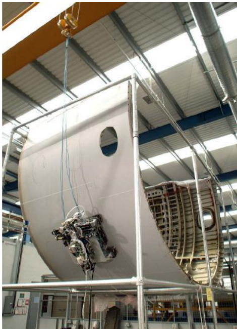
Fig. 11. Robot climbing on a D10 aircraft fuselage section
