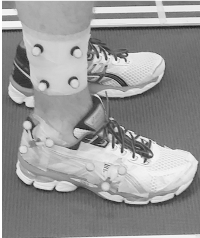
Figure 1 – Lateral view of a participant's lower leg and foot/shoe highlighting the rearfoot technical marker placement, an additional technical cluster is visible and located at the midshaft of the 5th metatarsal but was not utilised for this study
