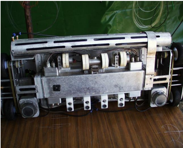
Figure 11: NDT Sensors On The Underside Of the ROBTANK Robot
