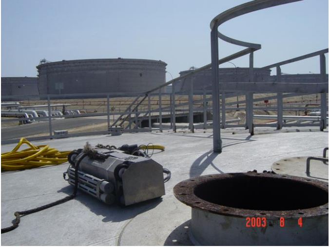
Figure 9: ROBTANK Floor And Wall-Climbing Robot For The Inspection Of Petrochemical Storage Tanks
