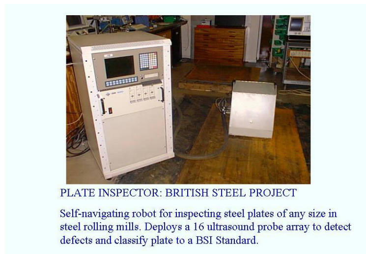
Figure 7 - Plate inspection robot which self navigates itself round the entire surface area of metallic plates of arbitrary size when initially located on a near one edge. Designed originally for deployment in steel rolling mills
