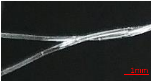
Fig. 3. Optical Images of two 200 \mu\text{m} cellulose tubes arranged in a double helix pattern.
