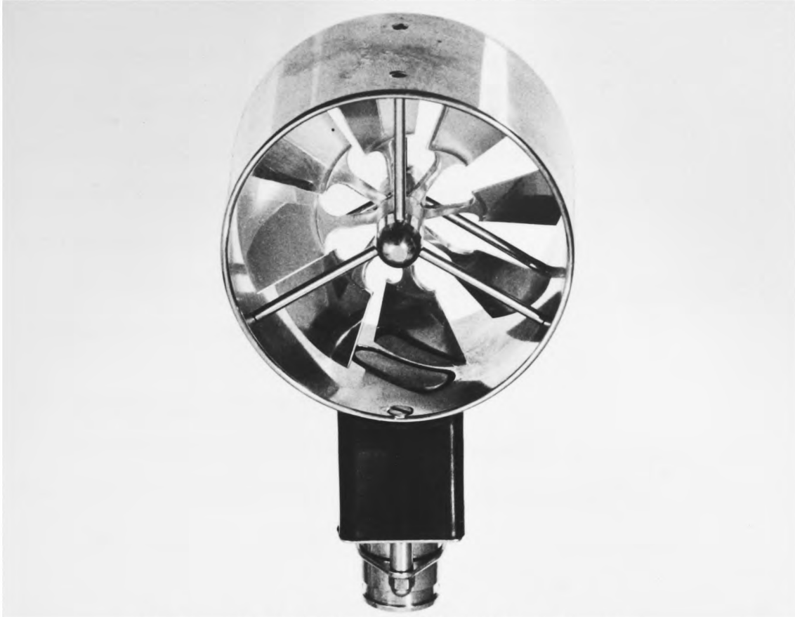
Fig. 3.2.a Rotating vane anemometer with capacitance change transducer (vane angle 40°, dimensions as for fig. 2.1.a)
