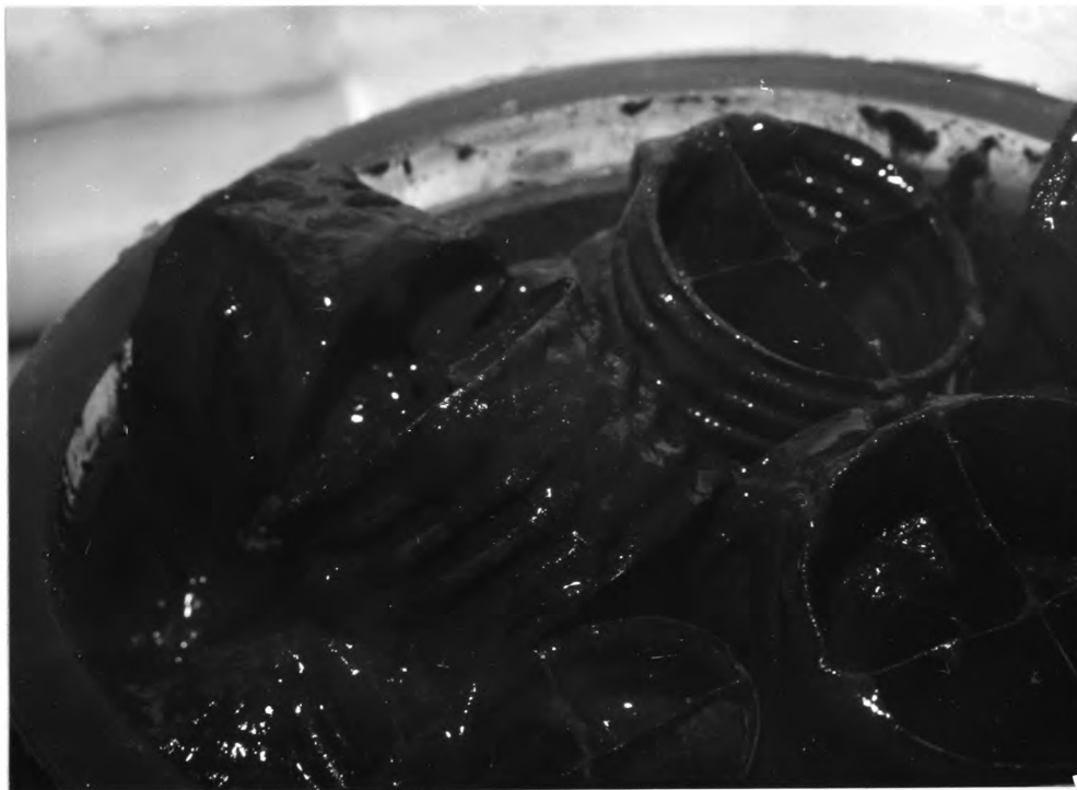
Plates 1 and 2. The Appearance of the Upflow Anaerobic Filter Support Rings on Day 166 (When the Filter was Dismantled). The associated slime layers may be distinguished
