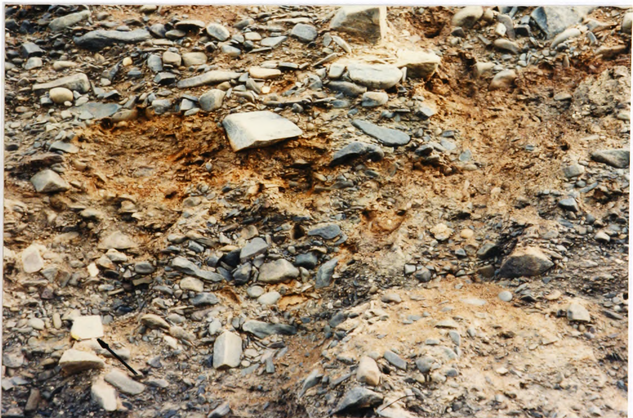
PLATE 7.10 Chng. 39 + 00, close-up of till material (50mm tape measure for scale)
