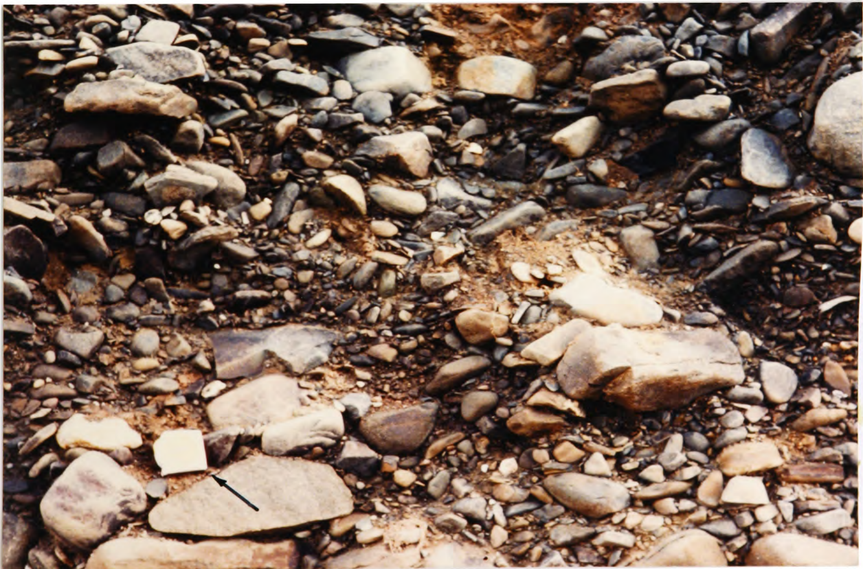
PLATE 7.8 Chng. 37 + 00, close-up of till material (50mm tape measure for scale)
