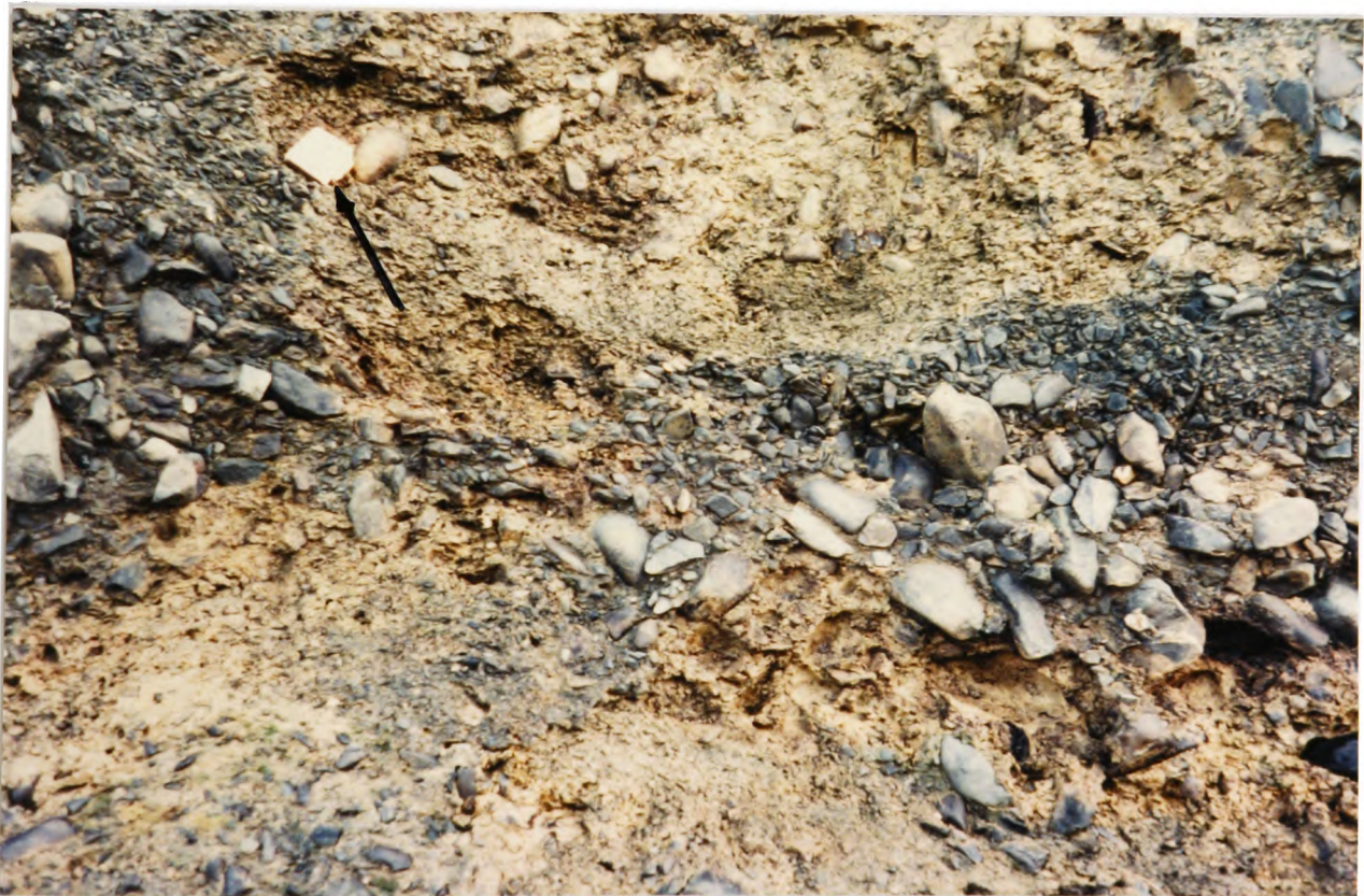
PLATE 7.12 Chng. 47 + 00, close-up of till material (50mm tape measure for scale)
