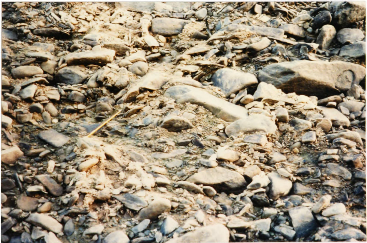
PLATE 7.18 Chng. 89 + 00, close-up of till material ( 15cm pencil for scale )
