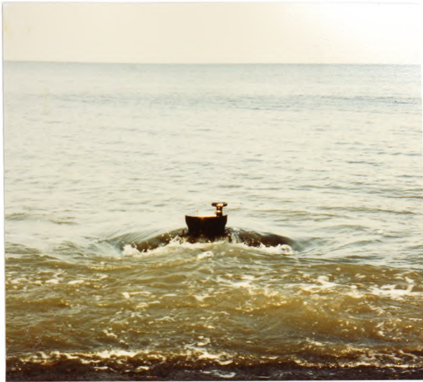
PLATE 9.1 Swash transducer at Aberarth (Feb 85)
