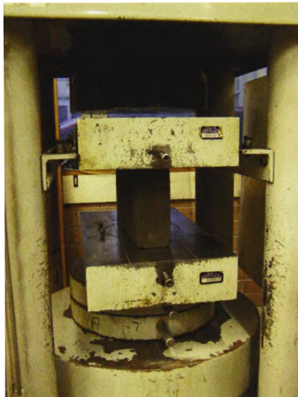
Figure 4.13: Using a Hounsfield testing machine used for the determination of the UCS was carried out on formulated unfired brick
