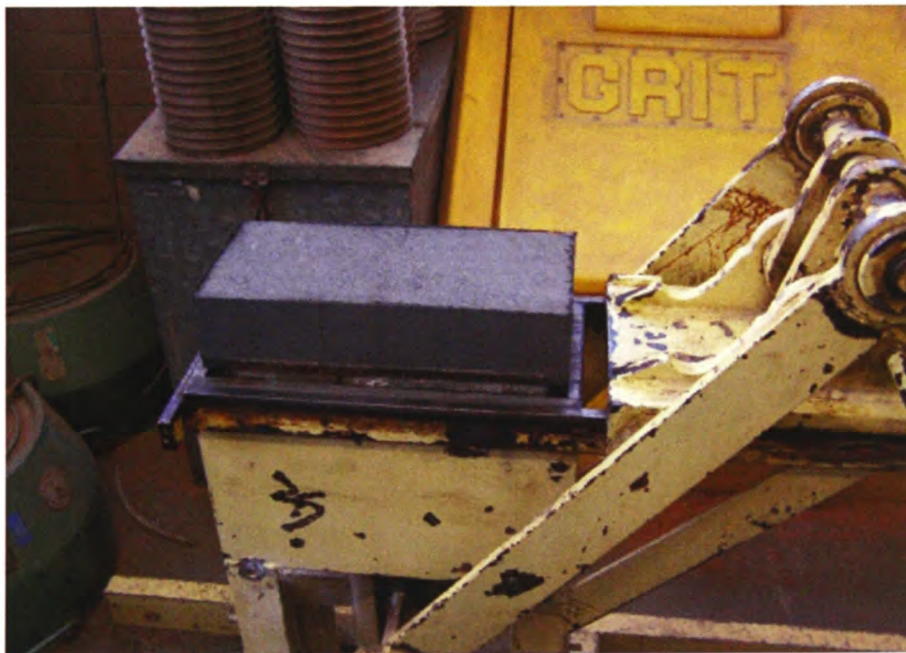
Figure 4.11: Unfired LOC-PFA brick freshly extruded from the steel mould
