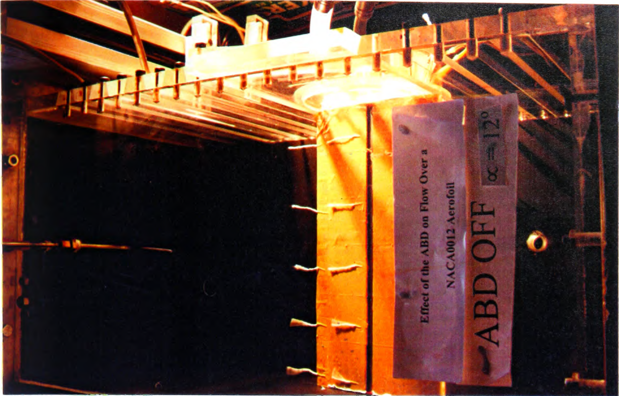
Figure 4-33 Flow visualisation using tufts over an aerofoil, \alpha=12^\circ .
