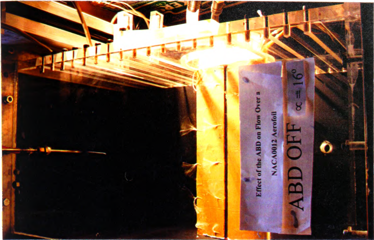
Figure 4-37 Flow visualisation using tufts over an aerofoil, \alpha=16^\circ .
