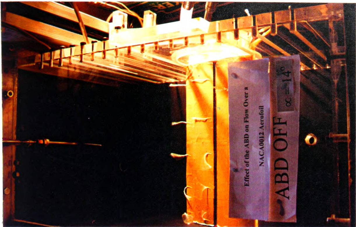
Figure 4-35 Flow visualisation using tufts over an aerofoil, \alpha=14^\circ .
