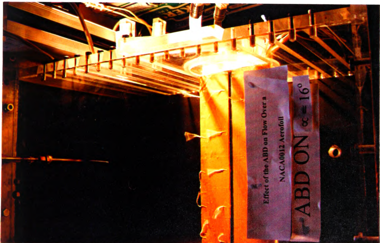
Figure 4-38 Flow visualisation using tufts over an aerofoil, \alpha=16^\circ .
