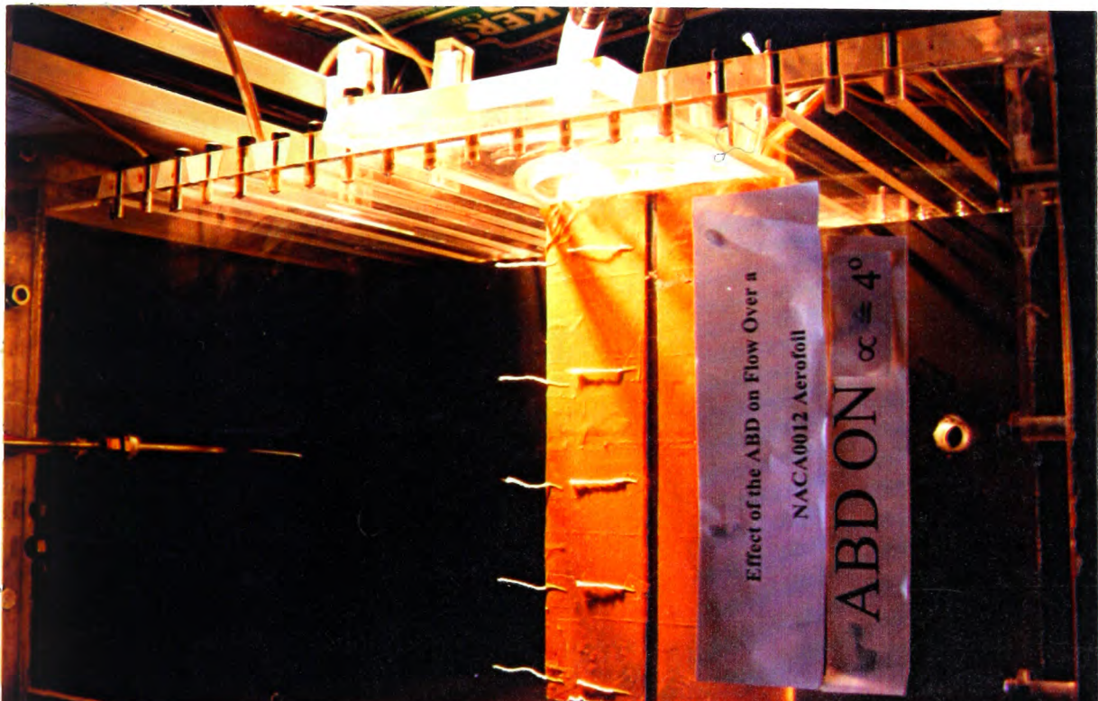
Figure 4-30 Flow visualisation using tufts over an aerofoil, \alpha=4^\circ .
