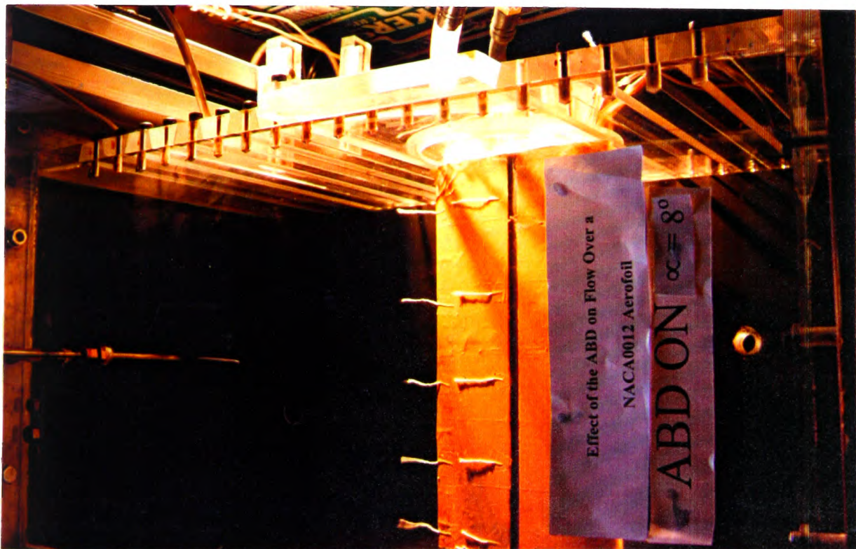
Figure 4-32 Flow visualisation using tufts over an aerofoil, \alpha=8^\circ .
