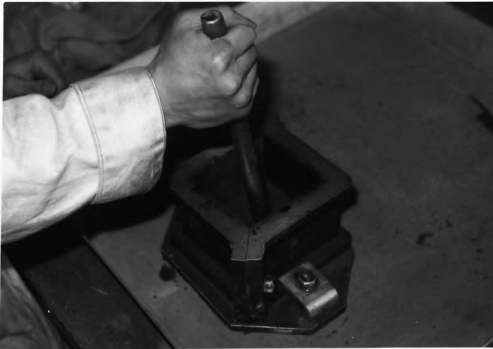
Plate 5.8 Hand-compacted in 5 equal layers of soil cement
