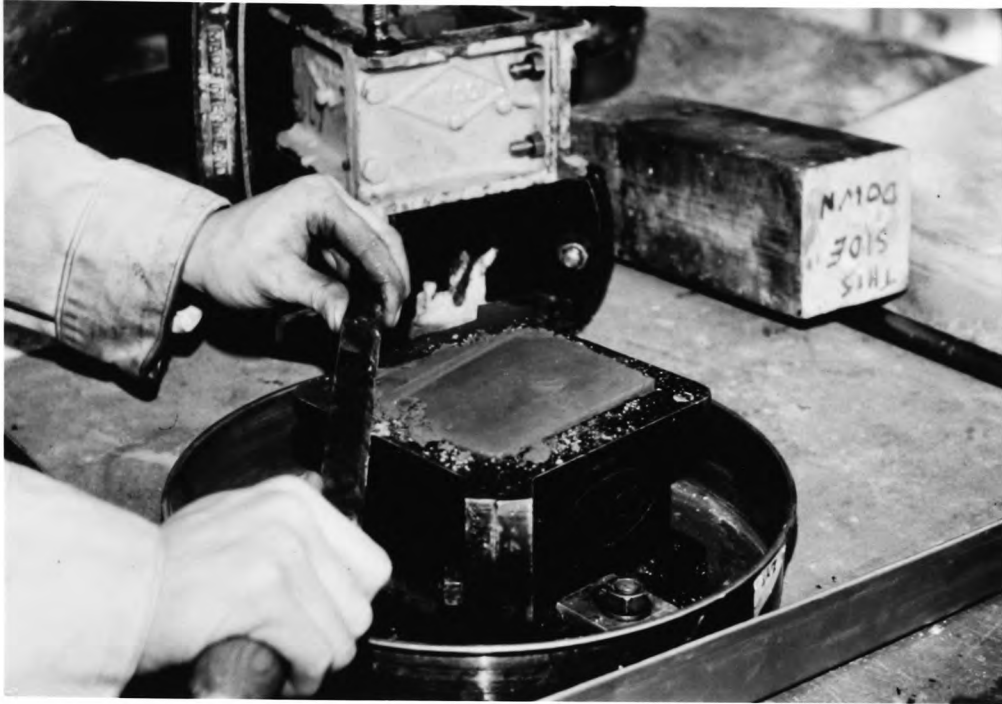
Plate 5.11 Level off a soil-cement cube
