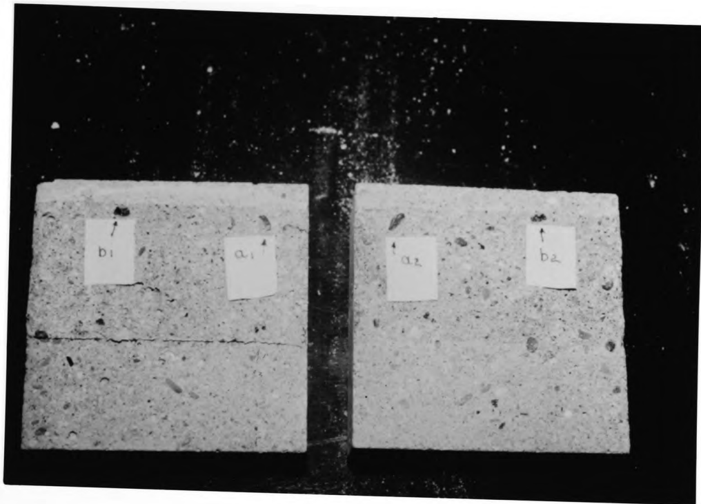
Plate 5.5 Typical fracture surface of a cube a_1 and b_1 correspond to the shear particles a_2 and b_2
