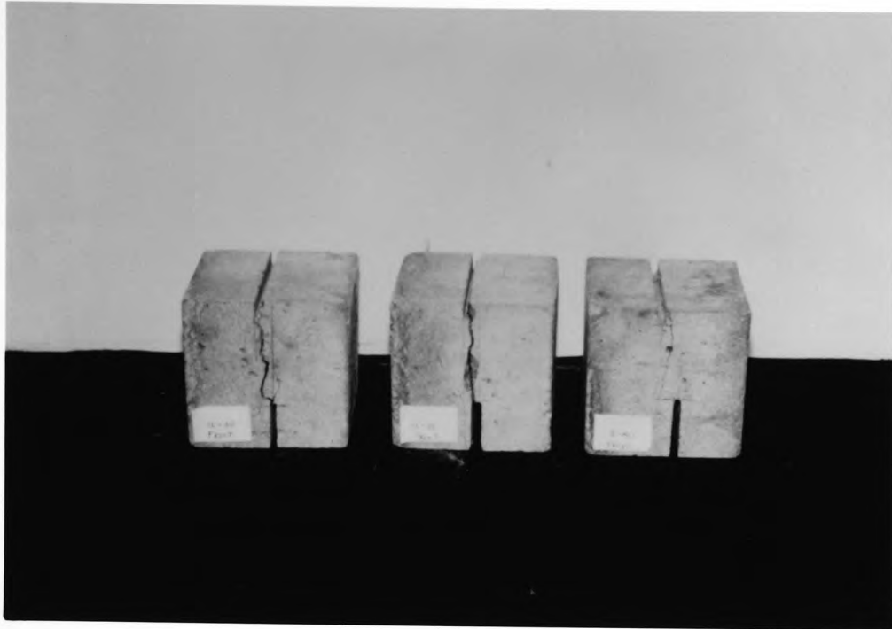
Plate 5.7 Typical single shear failure patterns of mortar cubes of a = 30 , 35 and 40\text{mm}
