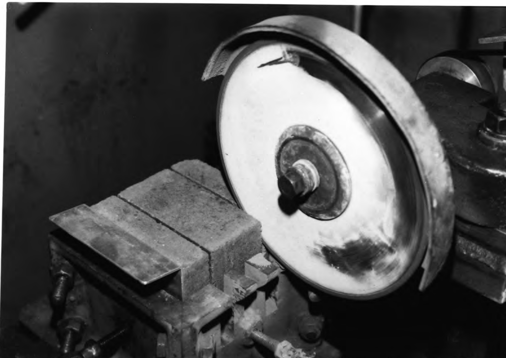
Plate 5.12 Insertion of notches on soil-cement cubes using a specially mounted circular lathe
