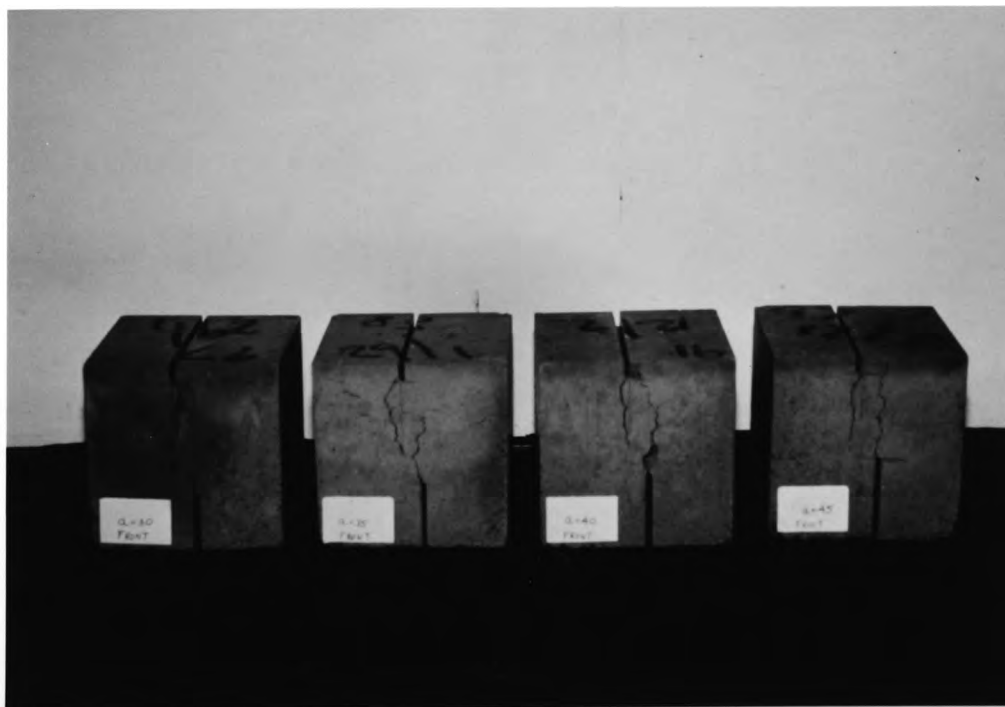
Plate 5.14 Typical single shear failure patterns of soil-cement cubes of a=30,35,40 and 45\text{mm}
