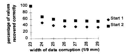
Fig. 4.2 Data Recovery within a DDS Basic Group in the Presence of a Lateral Corruption
