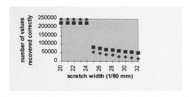
The coding between synchronizations is small enough to appear between deinterleaved errors when Nb is 4 or 8 and so allows a significant proportion of values to be recovered correctly.
