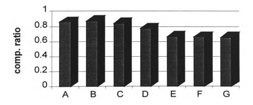
Fig. 3.1 Relative Performance of the Rice Algorithm (comp. ratio = output size/input size)
