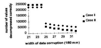
Fig. 4.1 Data Recovery within a DDS Basic Group in the Presence of a Longitudinal Corruption
