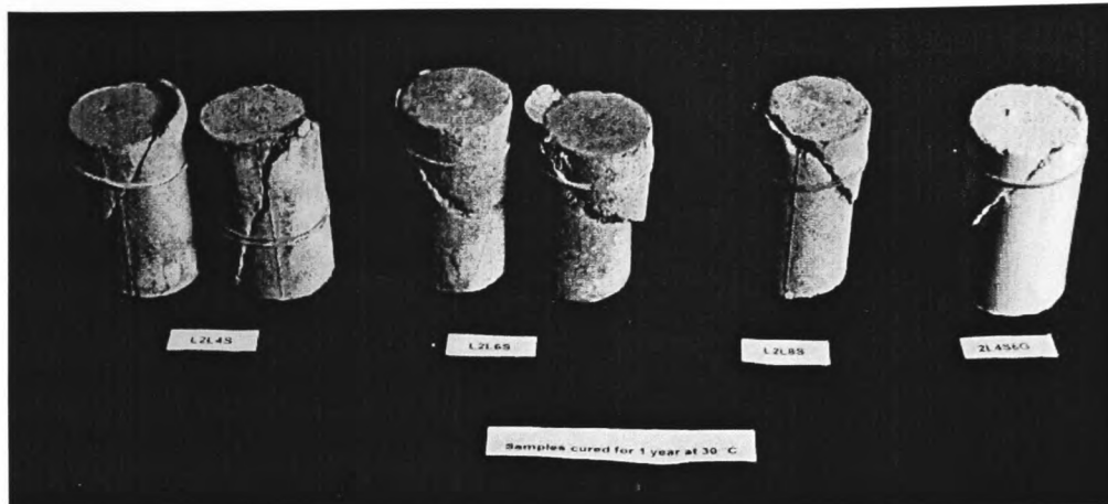
Figure 7.49 Failed specimens exhibiting shear failure plane after a curing period of 1 year at 30 °C
