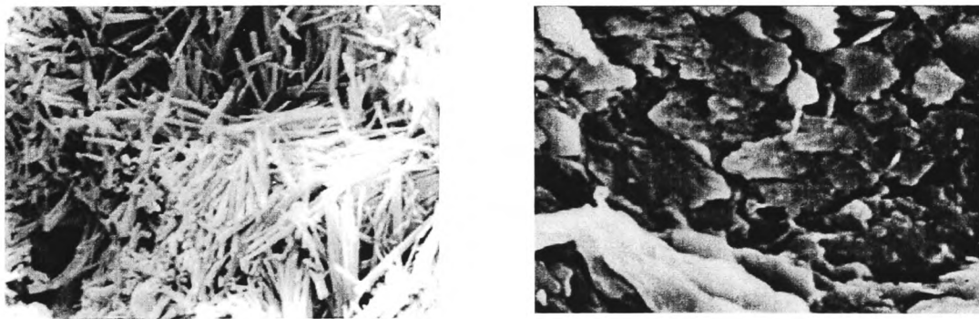
Figure 8.2 SE micrographs of the lime-stabilised layer ① (left) and the unstabilised layer ② (right)
