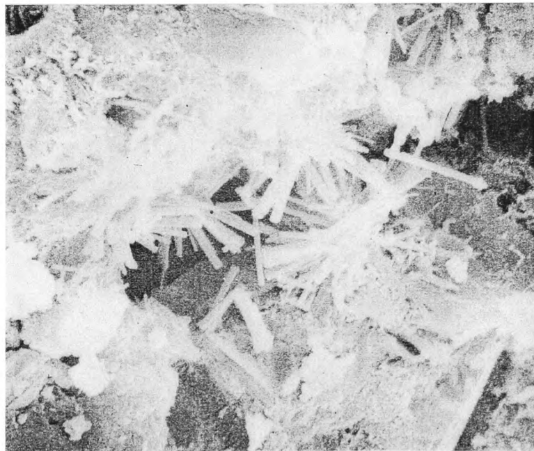
Figure 7.43 Expansive crystals on a sample consisting of 50% ggbs and 50% gypsum after 7 days of moist curing at 30 °C and subsequent soaking for 20 weeks (x2000)
