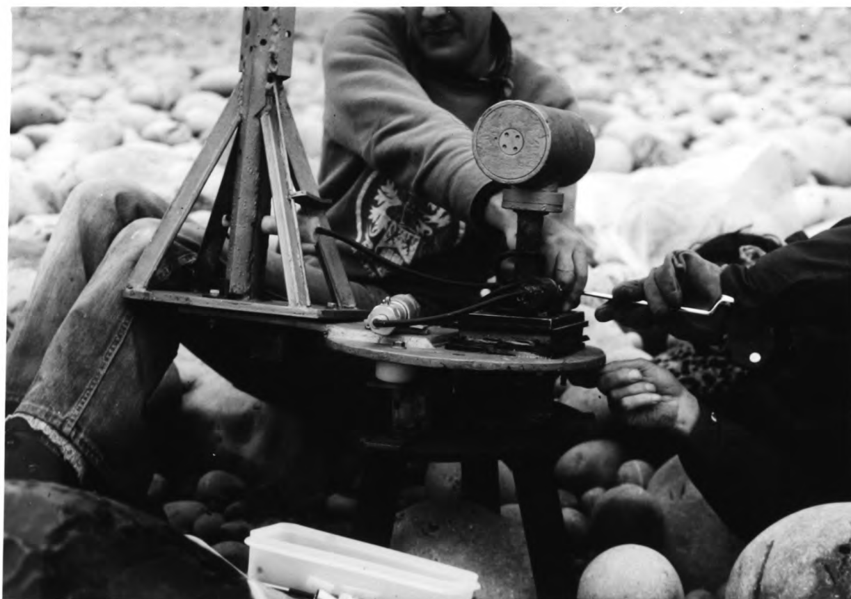
PLATE 18 Bolting the Swash Transducer into position.
