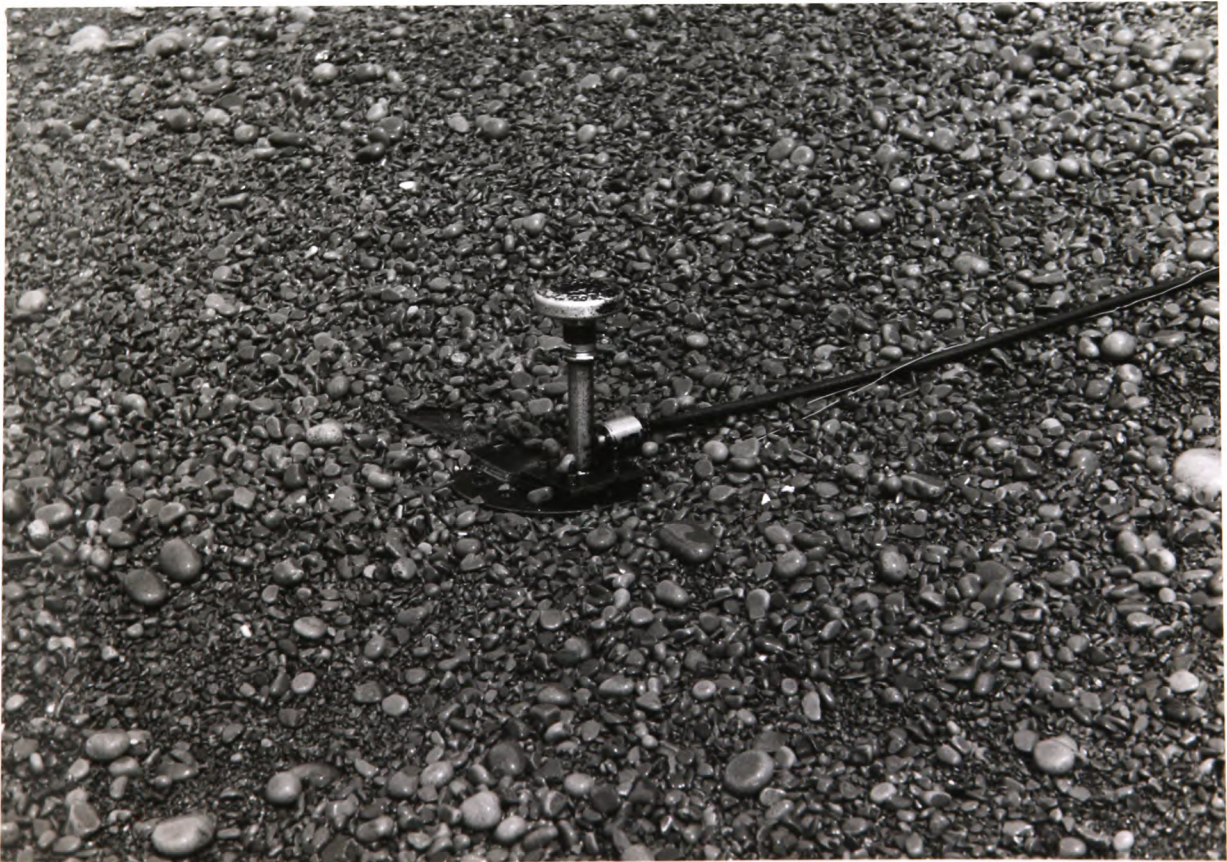
PLATE 22 Mark II swash transducer on beach (9.5.81)
