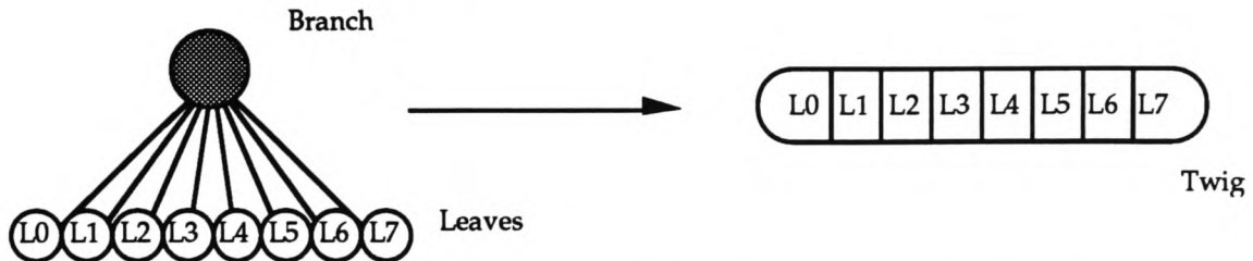
Figure 3.5 - Shows how a branch and its connected leaves can be replaced by a single entity.
