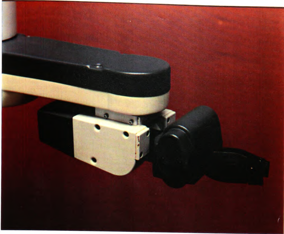
Plate A4.3 - The RTX's end effector, before it was modified to carry a camera.
