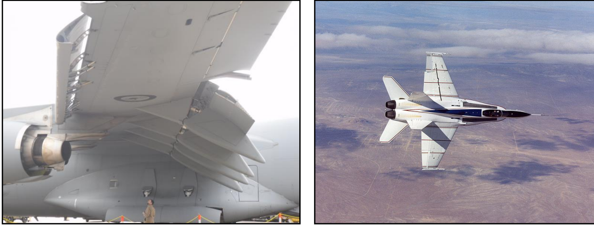
Fig. 2. Deployed high-lift devices in an RAAF Boeing C-17 Globemaster III (left) and McDonnell Douglas F/A-18 Hornet (right). Photos: Marques Aviation Ltd; Jim Ross (NASA).
