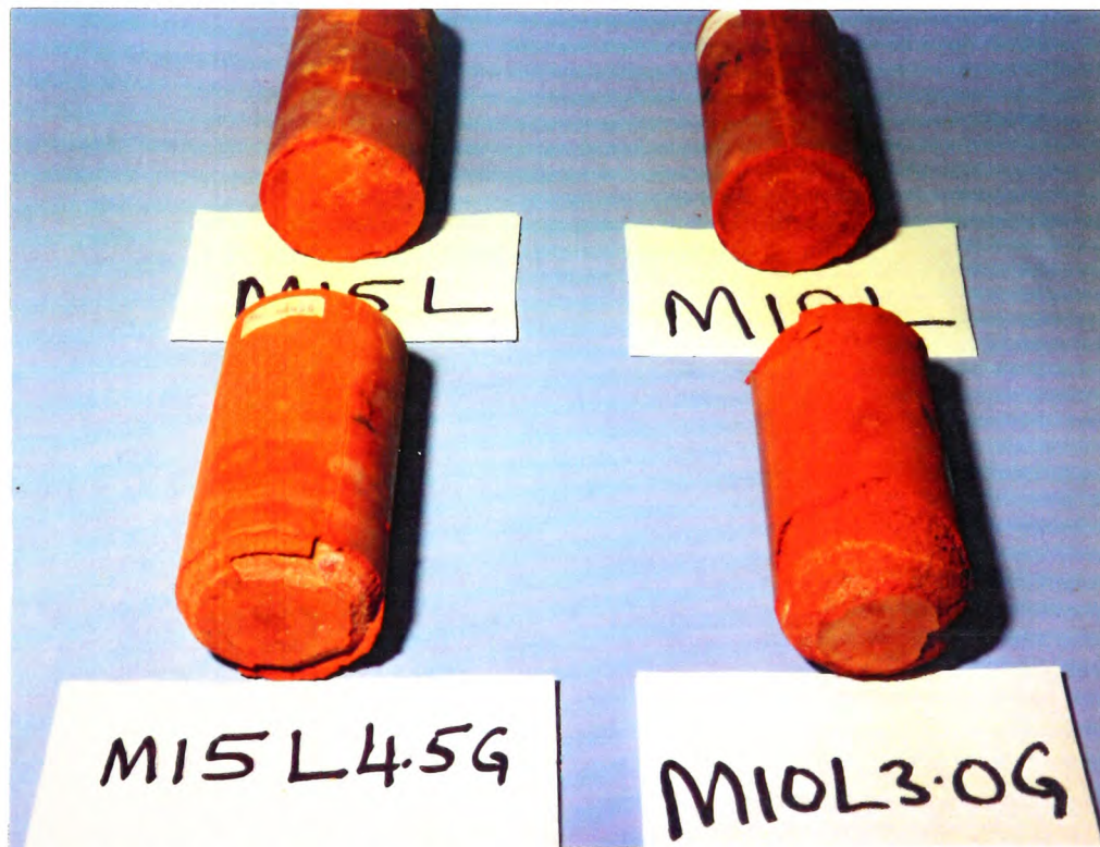
Plate 6.2 Murram-lime and murram-lime-gypsum samples subjected to 14 cycles of (a) full and (b) partial wetting and drying.
