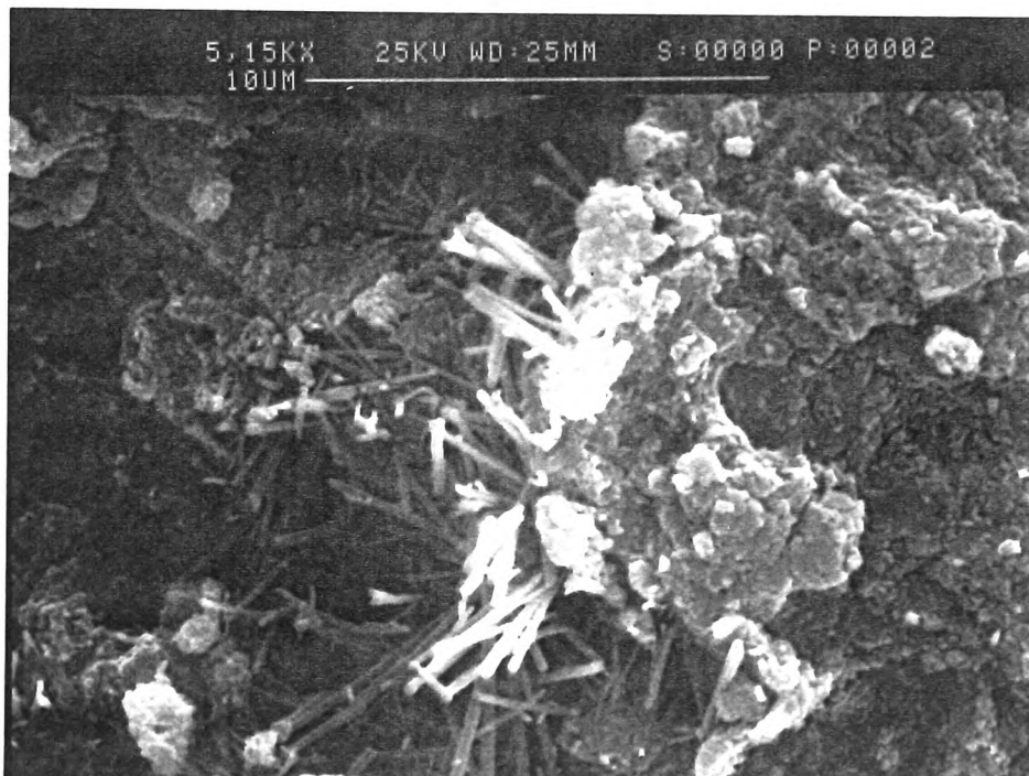
Plate 6.5 Scanning electron micrograph of murrum-15wt% lime-4.5wt% gypsum cured for 4 weeks at 30°C.
