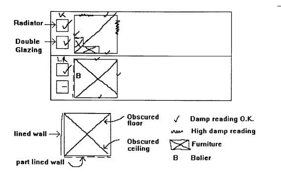
Figure 25. Completed Room Notation with Key to Annotations. Source: Halifax Plc.
