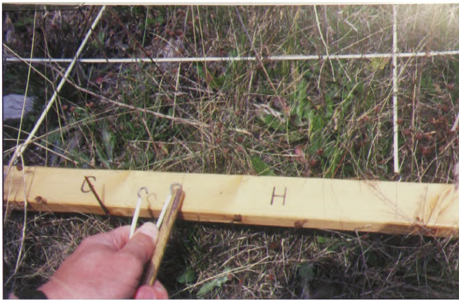
Plate 3.1 The dividing wire is hooked onto the end of the cane.
