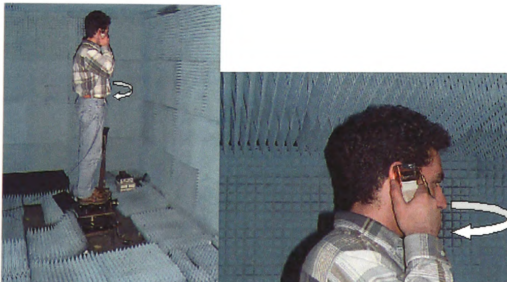
Fig. 4.34 Settings for radiation patterns measurements in the presence of the operator.
