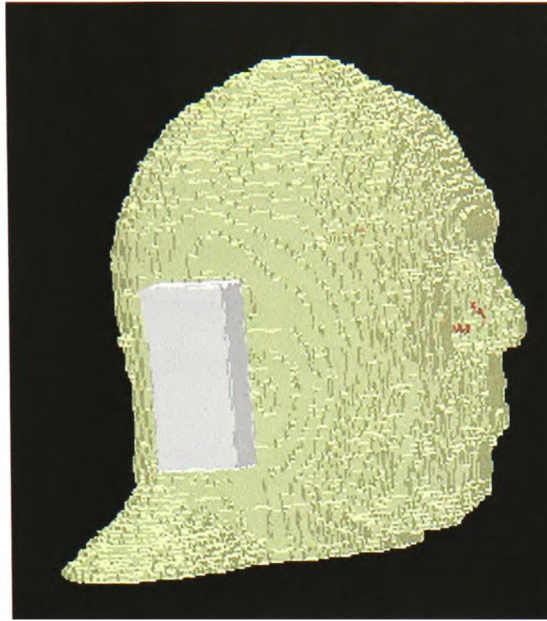
Fig. 4.35 The FDTD numerical head/shoulders model and handset used for far-field radiation pattern evaluation.
