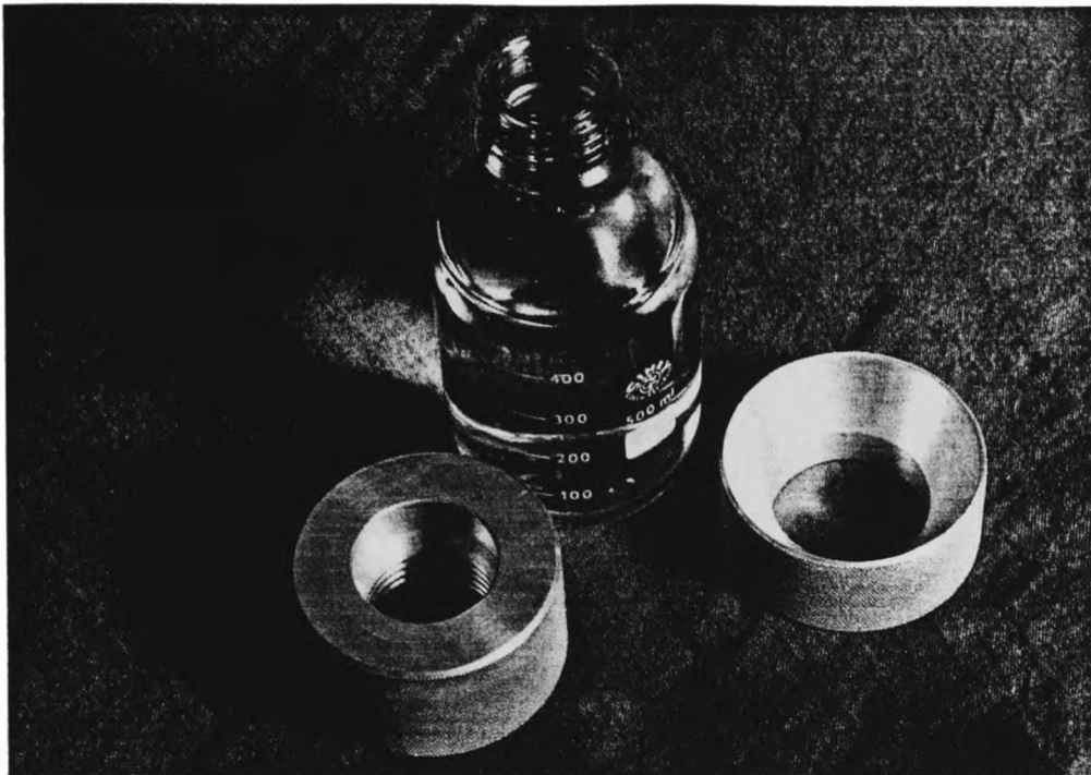
Fig.2. 28 500 cm 3 sample bottle and aluminium collars
