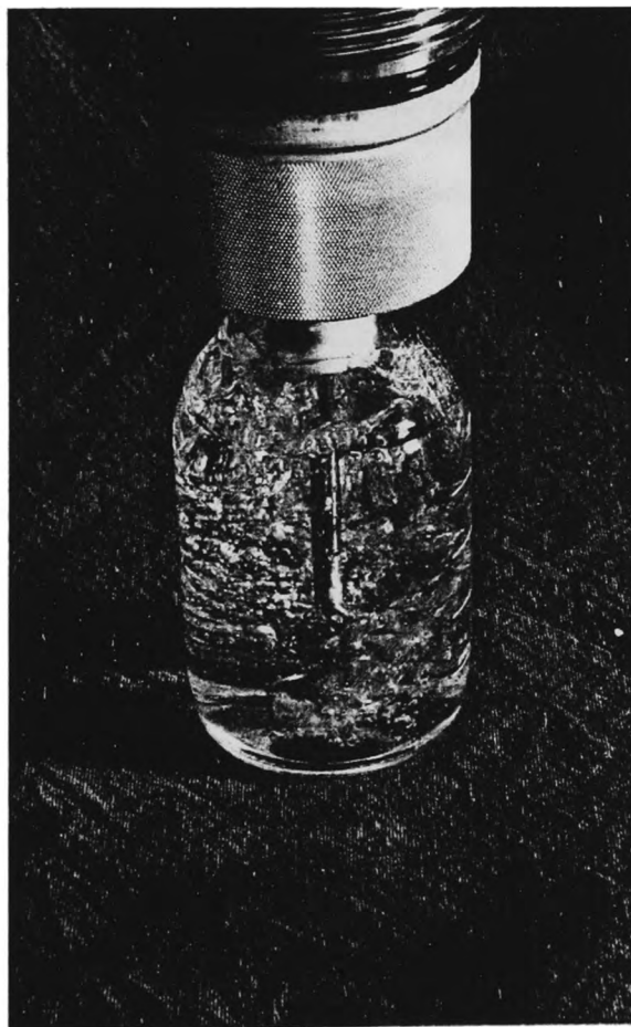
Fig.2. 29 Sample bottle, with aqueous sample, showing the vortex action of the incoming CO 2
