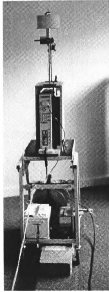
Figure 4-10: Omnidirectional antenna mounted on the mobile trolley for measurements at 11 GHz
