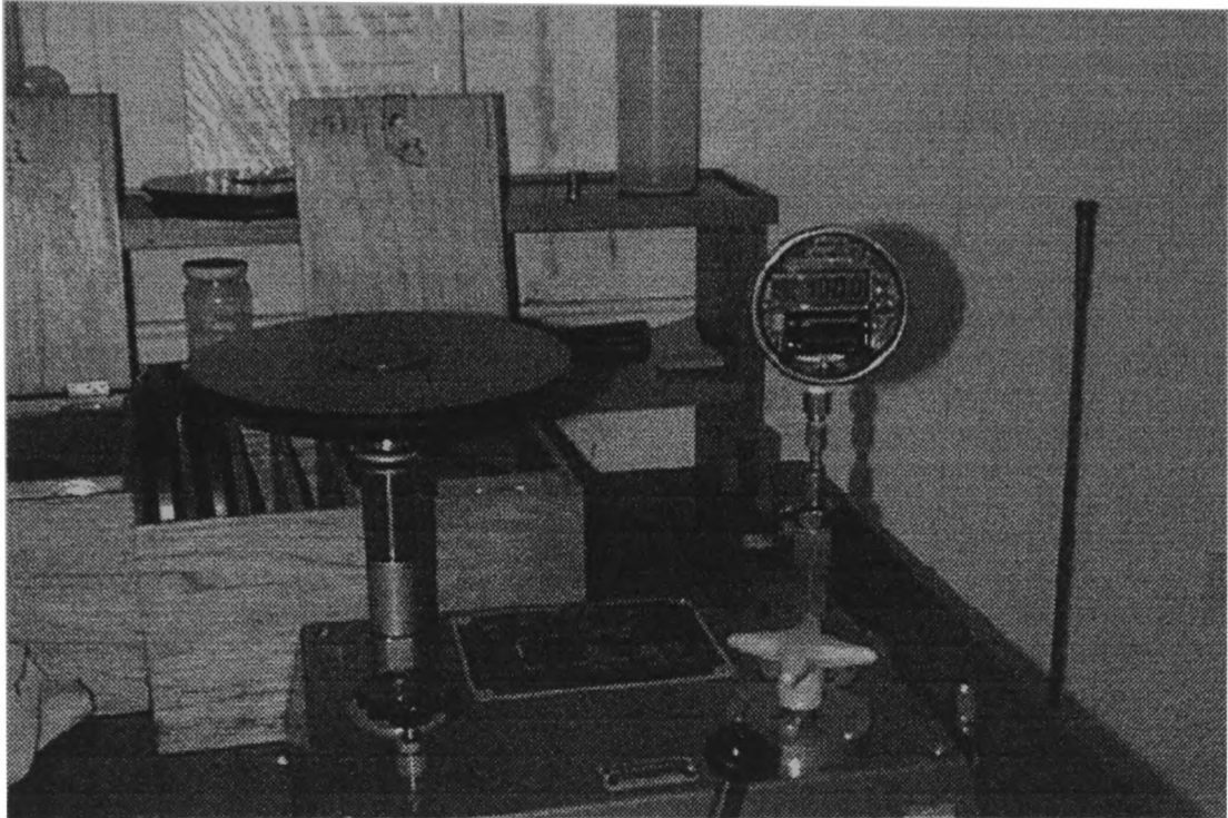
FIGURE 5: Testing the accuracy of the digital pressure gauge on a dead weight tester.
