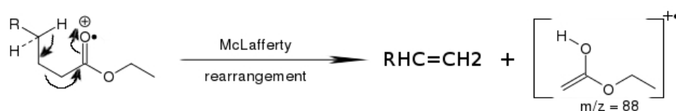
Figure 6.6: McLafferty rearrangement of a FAEE and the formation of a 88 Da fragment.
