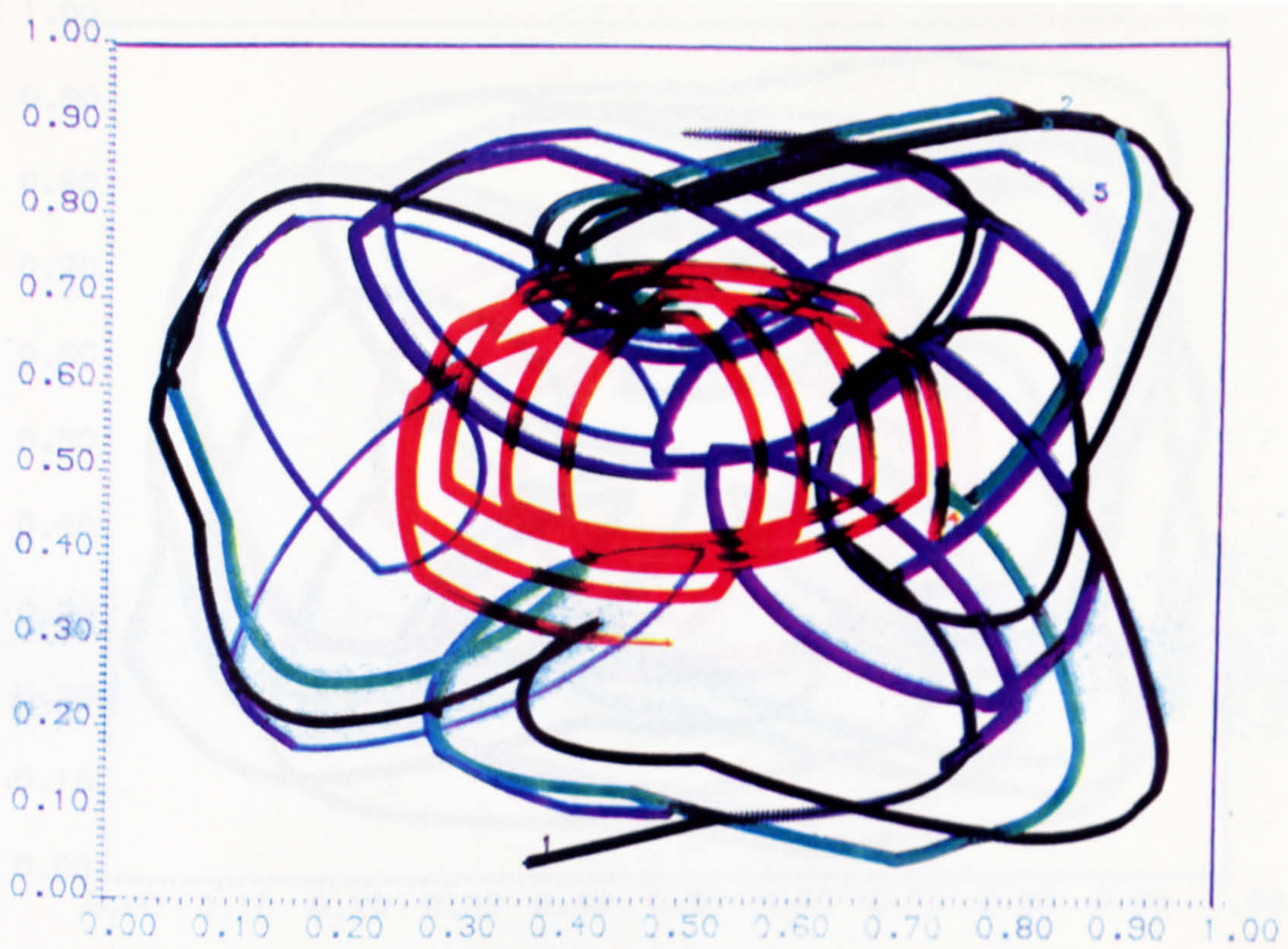
Figure (5.72) Particle mixing for a pseudoplastic fluid at Re=1 , T=2s , time 60s, 4 walls in discontinuous co-rotational motion.
