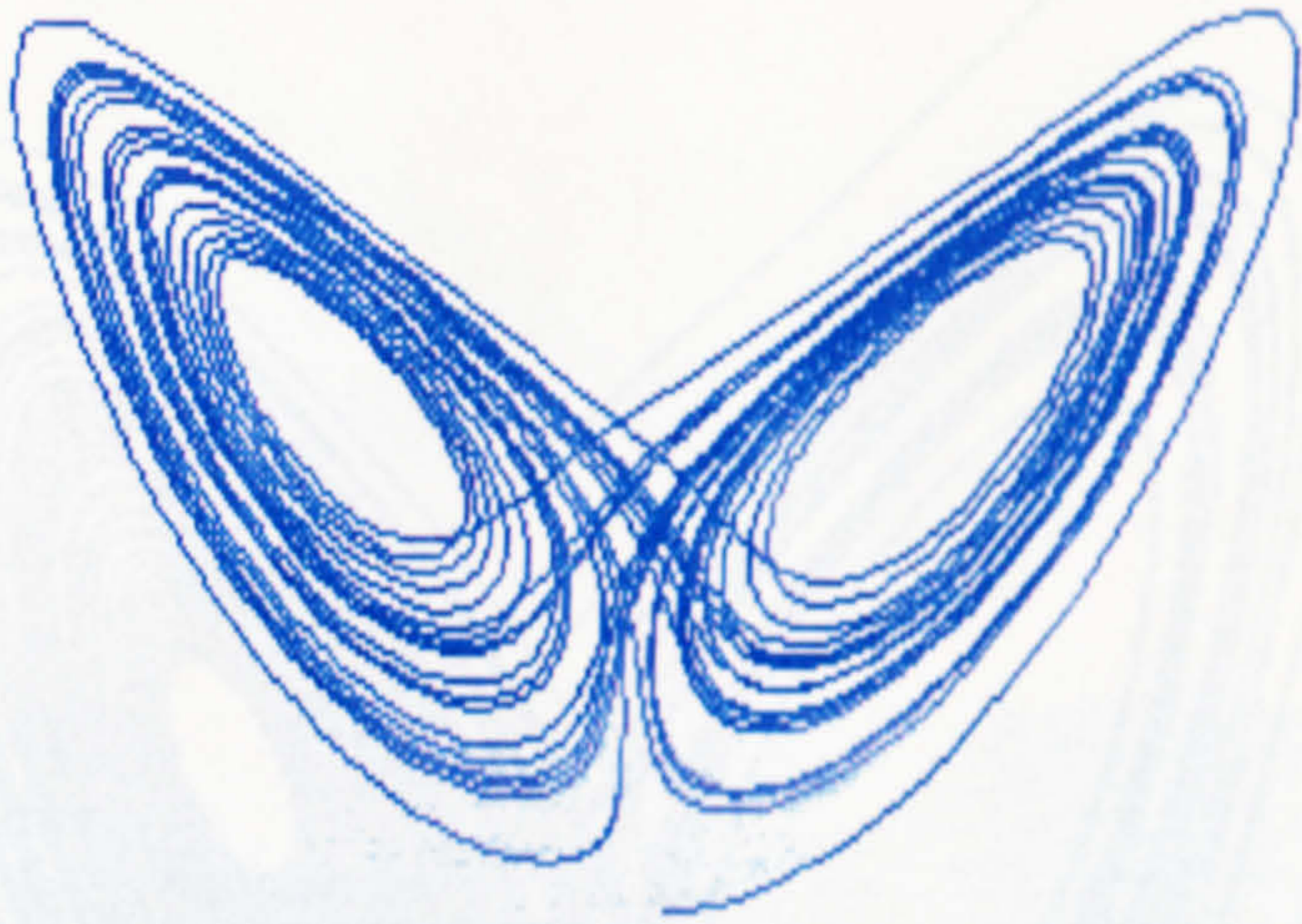
Figure (8.6) The chaotic attractor of a pseudoplastic fluid at r=18.12 , time =30 seconds. Scale: -30 < X < 30 , 0 < Z < 60
