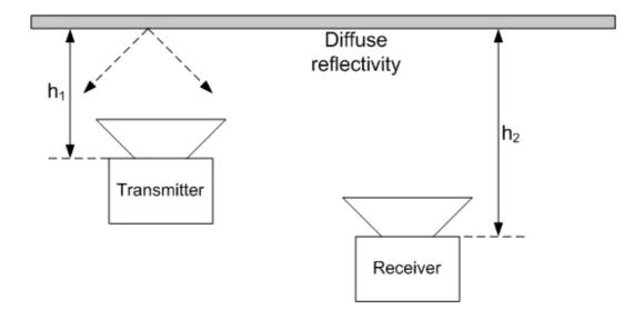
Figure 6-1: Non-directed non-line of sight LOS (Diffuse) configuration.
