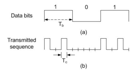
**Figure 1-1:** Encoding in optical CDMA (a) data bits '101' (b) transmitted sequence 10010 for bit '1'
