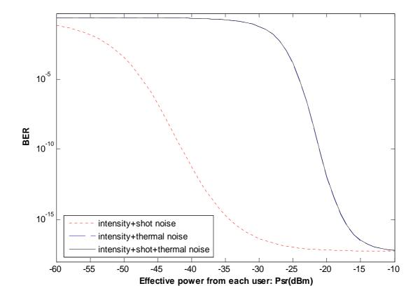
Figure 4-8: BER versus effective power P when number of active users is 43.
