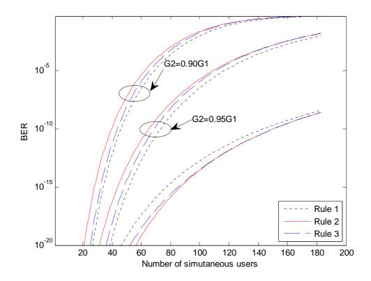
Figure 3-2: BER probability for I = 14 and splitter loss of 0.5 dB.
