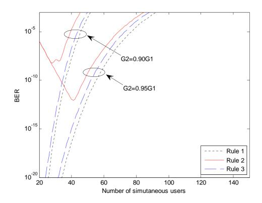
Figure 3-8: BER probability for w = 14 and splitter loss of 1.0.dB.
