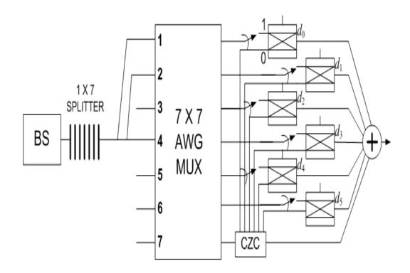
Figure 4-3: Encoder for SAC-OCDMA system based on PDC. (BS: Broadband Source)
