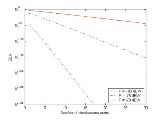
Figure 5-3: BER versus number of users for MCMLCs and w = 4.
