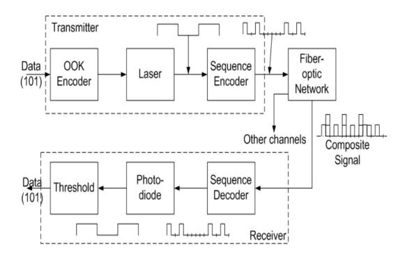
Figure 2-2: Transmitter and receiver model for FO-CDMA system.
