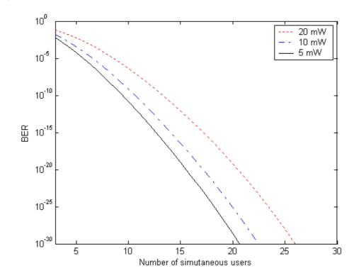
Figure 6-5: Error probability versus number of users for data rate of 2 Mbps.
