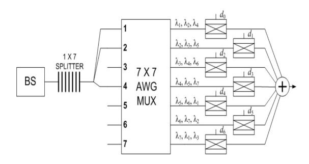
Figure 4-1: Encoder for PDC based SAC-OCDM system (BS: Broadband Source).
