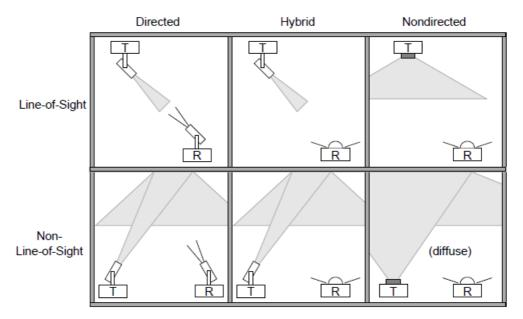
Figure 2-3: Classification of simple Infrared links (Reproduced from [72]).
