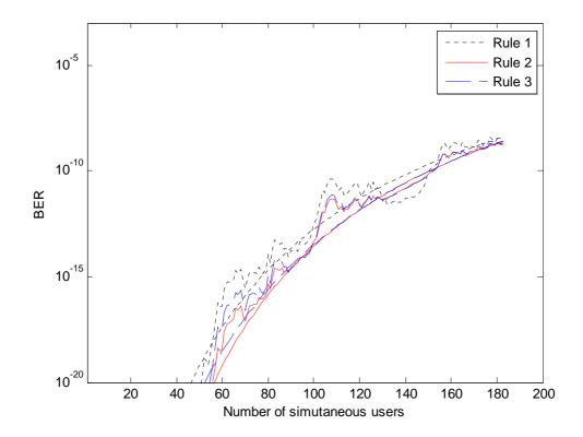
**Figure 3-5:** BER probability for w = 14 and splitter loss of 0.5 dB.
