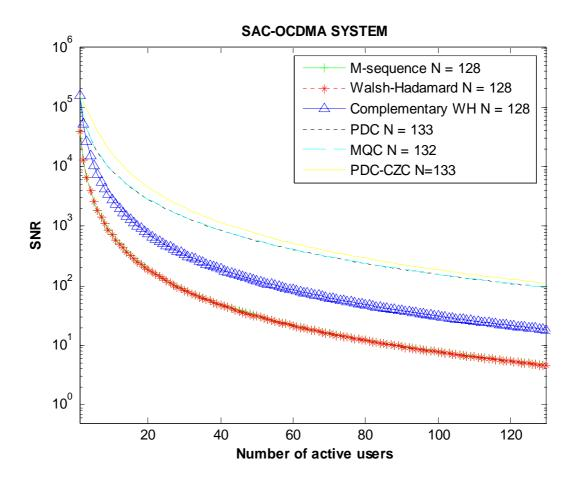
Figure 4-6: SNRs versus number of active users when P = -10 dBm.
