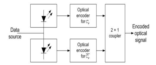
Figure 5-1: Structure of the MCMLC encoder.
