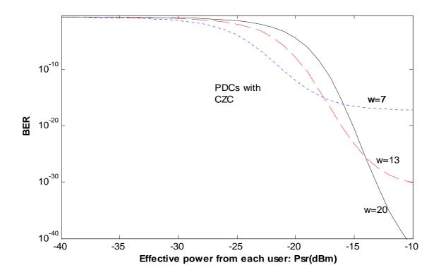
**Figure 4-9:** BER versus effective power P when number of active users is 43, taking into account the intensity noise, shot noise, and thermal noise.
