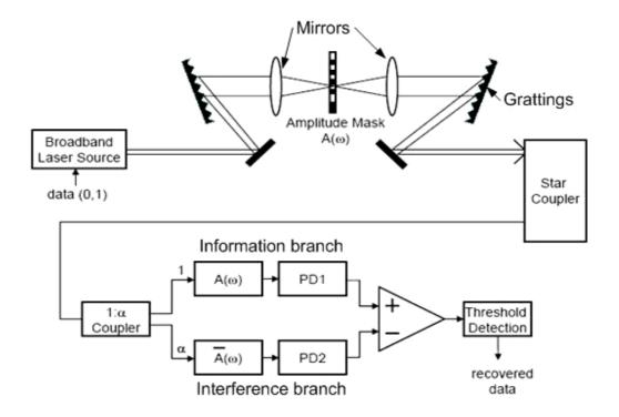
Figure 2-4: Basic Principle diagram of SAE/OCDM system (Reproduced from [50]).
