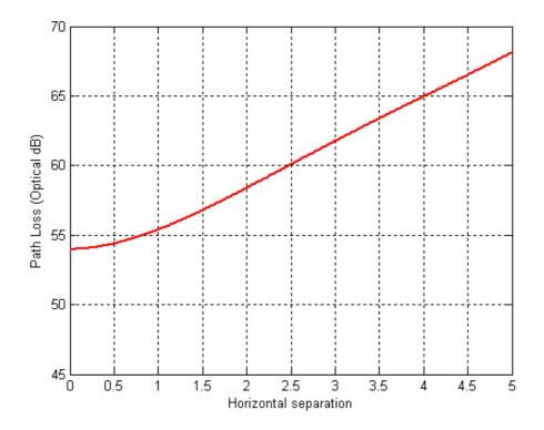
**Figure 6-2:** Optical path loss of a diffuse infrared links employing a Lambertian transmitter and a detector of area  $A_d = 1 \text{ cm}^2$  and reflectivity of 80% measured in a typical room.
