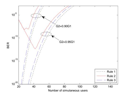
**Figure 3-7:** BER probability for w = 14 and splitter loss of 0.5 dB.
