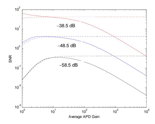
**Figure 3-3:** SNR versus the average APD Gain. Dotted curves are for fixed value of  $F_e = 2$ .
