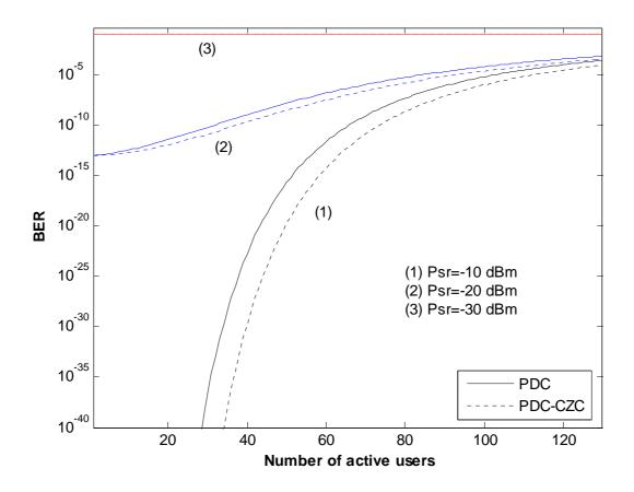
Figure 4-10: BER versus number of active users when effective power P is different.
