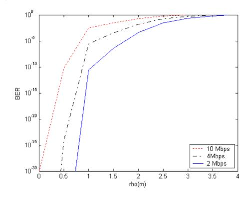
**Figure 6-4:** BER versus user's distance from base station  $(\rho)$  for various bit rates. Number of interferes is 5 and Pt = 20 mW.
