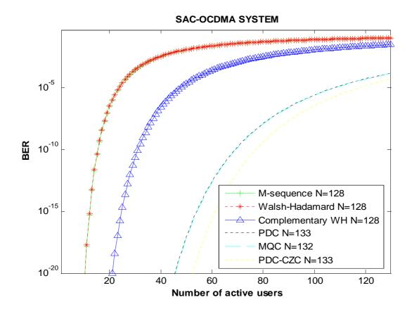
Figure 4-5: BER versus number of active users for different codes.
