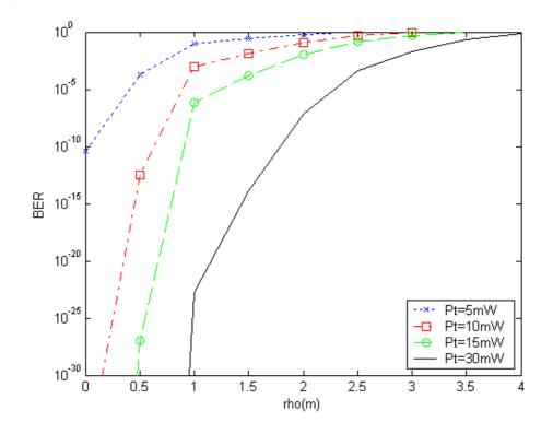
**Figure 6-3:** BER versus user's difference from base station  $(\rho)$  for various transmission powers. Number of interferes is 5.
