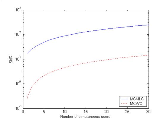
**Figure 5-4:** SNR versus number of users for MCMLCs for P = -70 dBW and w = 4.
