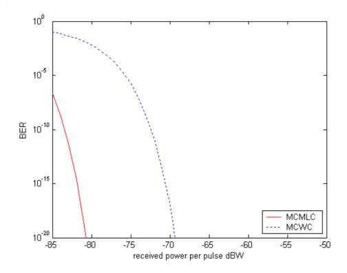
Figure 5-5: BER versus received power per pulse under full load for MCMLC and MCWC.
