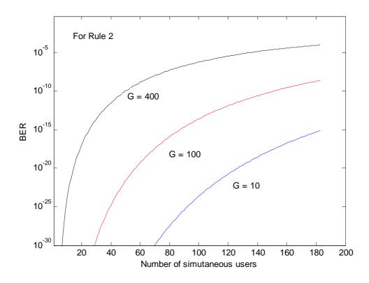
Figure 3-4: BER versus the number of simultaneous users for different values of APD Gain.
