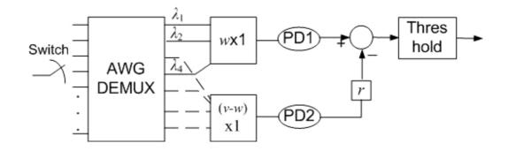
Figure 4-2: Decoder for PDC based SAC-OCDM system.
