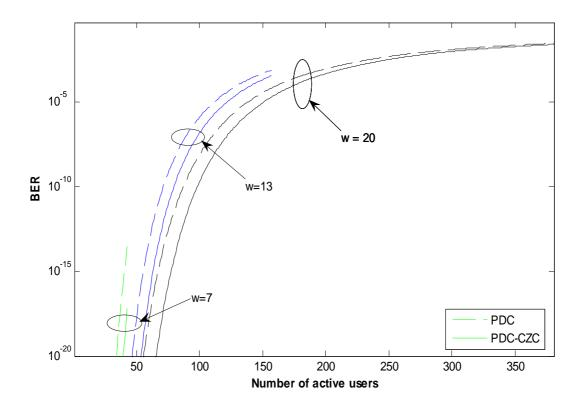
Figure 4-7: BER versus number of active users when P = -10 dBm.
