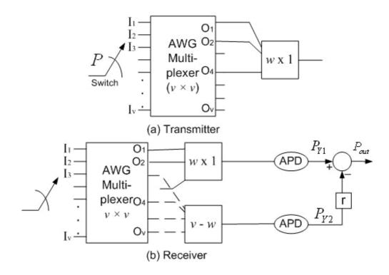
Figure 3-1: SAC-OCDMA system based on perfect difference codes [5].
