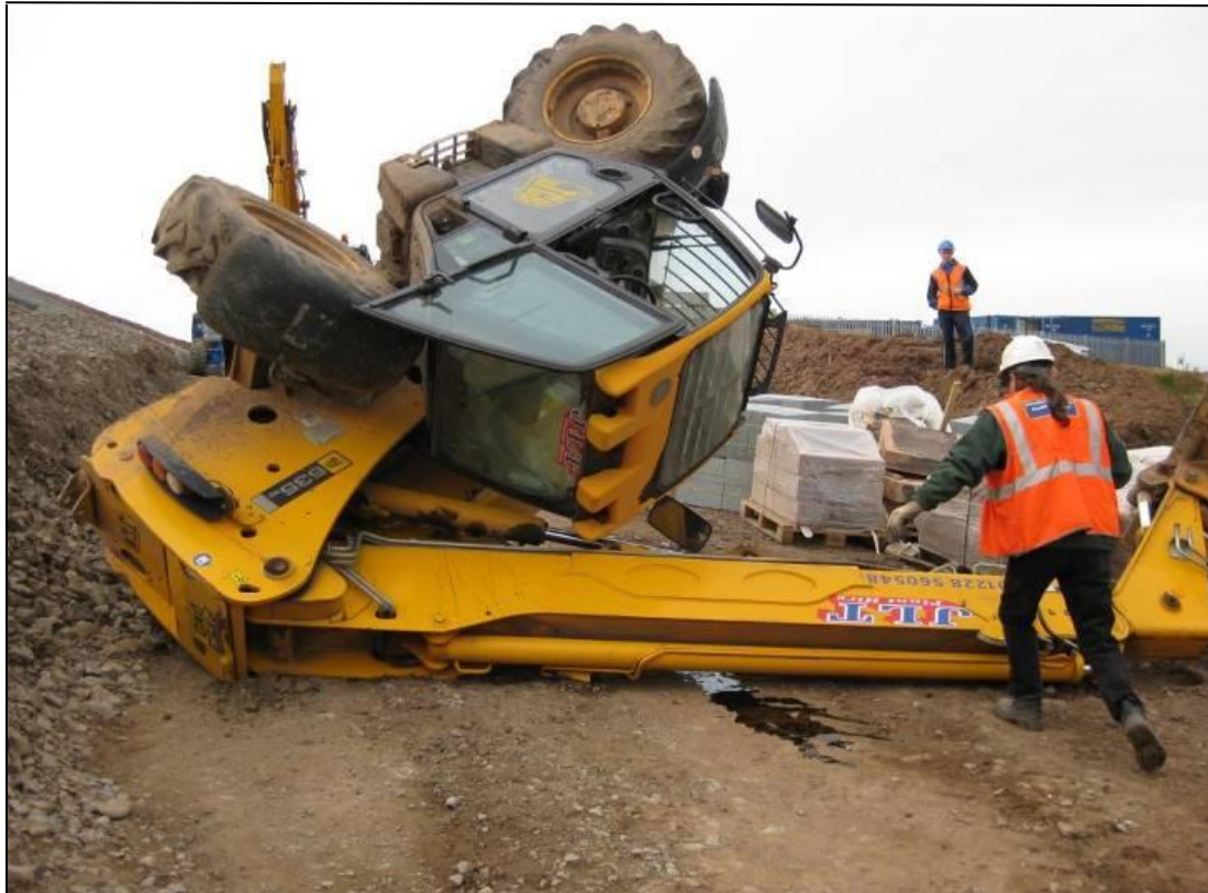
Figure 28: An overturned road rail machine 2011 (courtesy: Network Rail)
