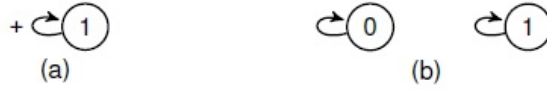
Fig. 4 (a) Interaction Graph of 1-variable Boolean function f(x) = x_1 and (b) BN state space of 1-variable Boolean function f(x) = x_1 .
