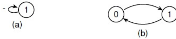
Fig. 8 (a) IG of 1-variable Boolean function f_1(x) = 1 and (b) BN of 1-variable Boolean function f_1(x) = 1 .
