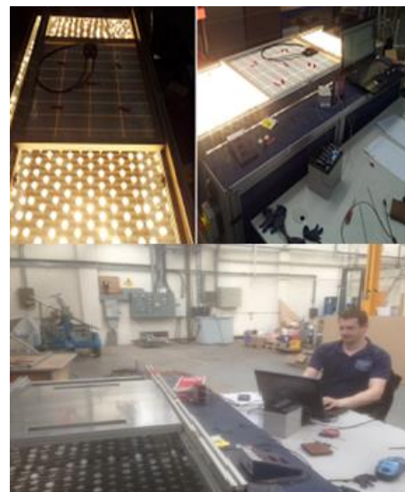
Fig.2. Laboratory setup and testing of PV module
