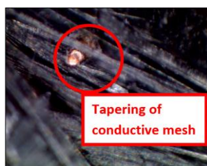
Figure 7. Tapering of conductive mesh
