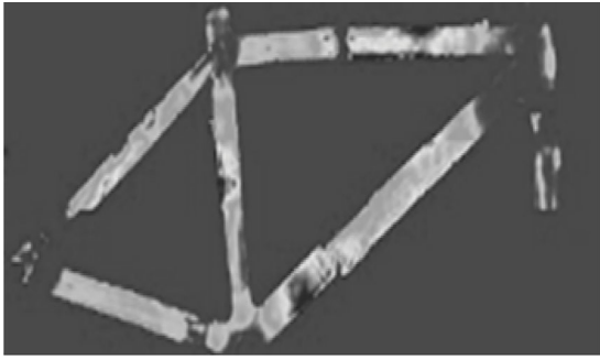
Figure 5. A broken frame showing signs of delamination.
