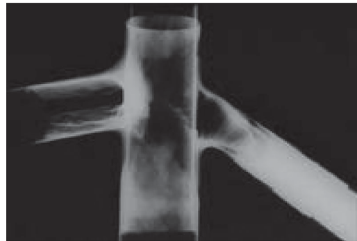
Figure 7. Damage in a CFRP bicycle component (Ning, 2015).
