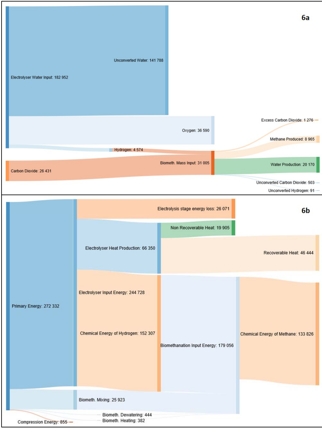
Figure 6 – Sankey Diagram of (6a) Mass Balance (kg / d) and (6b) Process Energy Inputs and Outputs (kWh / d)
