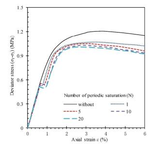
Fig. 2. Typical curves of deviator stress against axial strain from triaxial tests with different numbers of periodic saturation at stress level about 0.5 (b) Confining pressure  $\sigma$ 3=300 kPa
