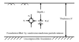
Fig. 8. A large-area foundation filled by sandstone-mudstone particle mixture subjected to periodic saturation
