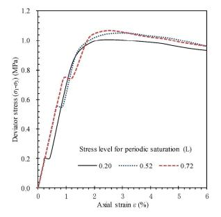
Fig. 3. Typical curves of deviator stress against axial strain from triaxial tests with periodic saturation for N=5 at different stress levels (b) Confining pressure  $\sigma$ 3=300 kPa
