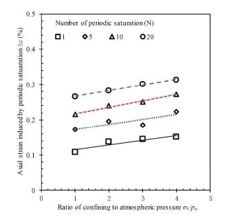
Fig. 7. Effects of confining pressure on increment of axial strain induced by periodic saturation (a) Stress level L=0.18 to 0.28 (mean 0.23)
