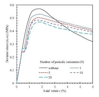
Fig. 2. Typical curves of deviator stress against axial strain from triaxial tests with different numbers of periodic saturation at stress level about 0.5 (a) Confining pressure  $\sigma$ 3=100 kPa
