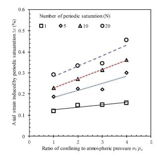
Fig. 7. Effects of confining pressure on increment of axial strain induced by periodic saturation (b) Stress level L=0.43 to 0.57 (mean 0.50)
