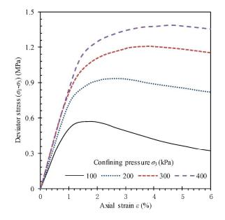
Fig. 1. Curves of deviator stress against axial strain from triaxial tests without periodic saturation 210x297mm (300 x 300 DPI)
