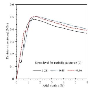
Fig. 3. Typical curves of deviator stress against axial strain from triaxial tests with periodic saturation for N=5 at different stress levels (a) Confining pressure  $\sigma$ 3=100 kPa
