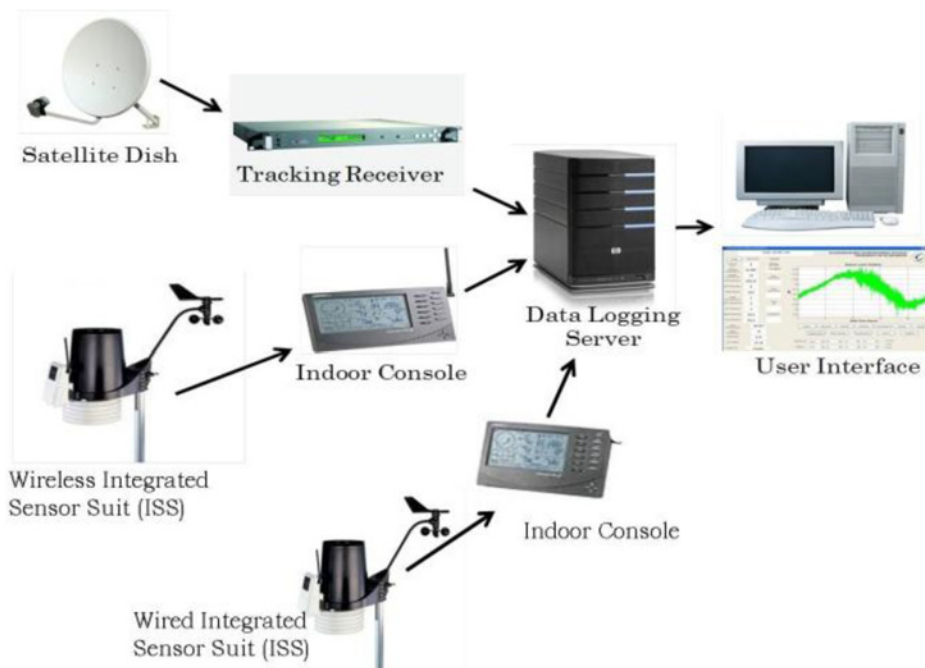
Fig. 4 Physical connectivity of complete satellite
