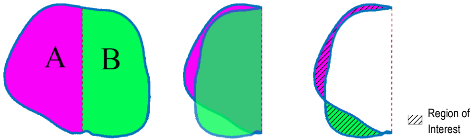
Figure 3.6. Computing the ROI. A typical Cross-section (left) was mirrored (middle), and the area corresponding to the region of interest (right) was computed
