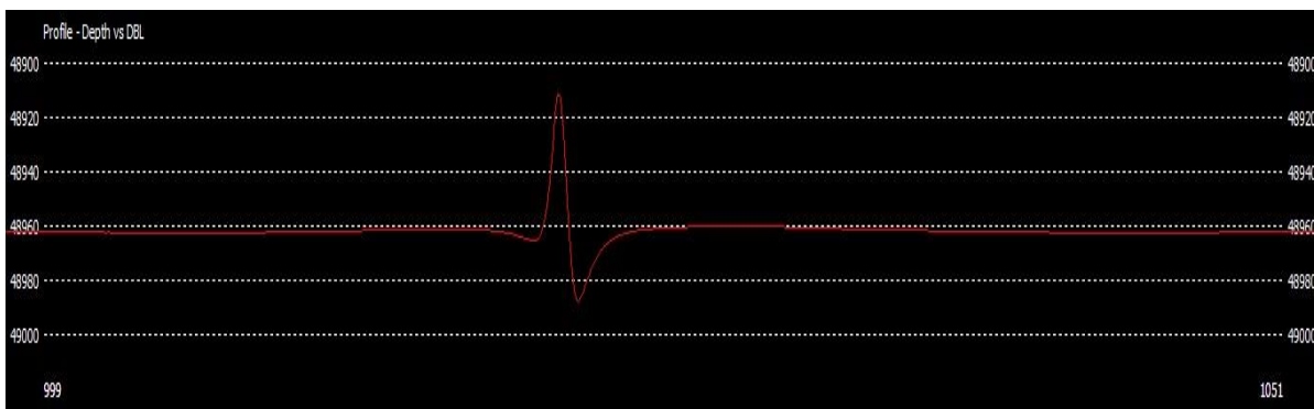
Figure 51. Example of a dipole from this study's magnetometer data set. This dipole has a reading of roughly 70nT (25 negative and 45 positive).
