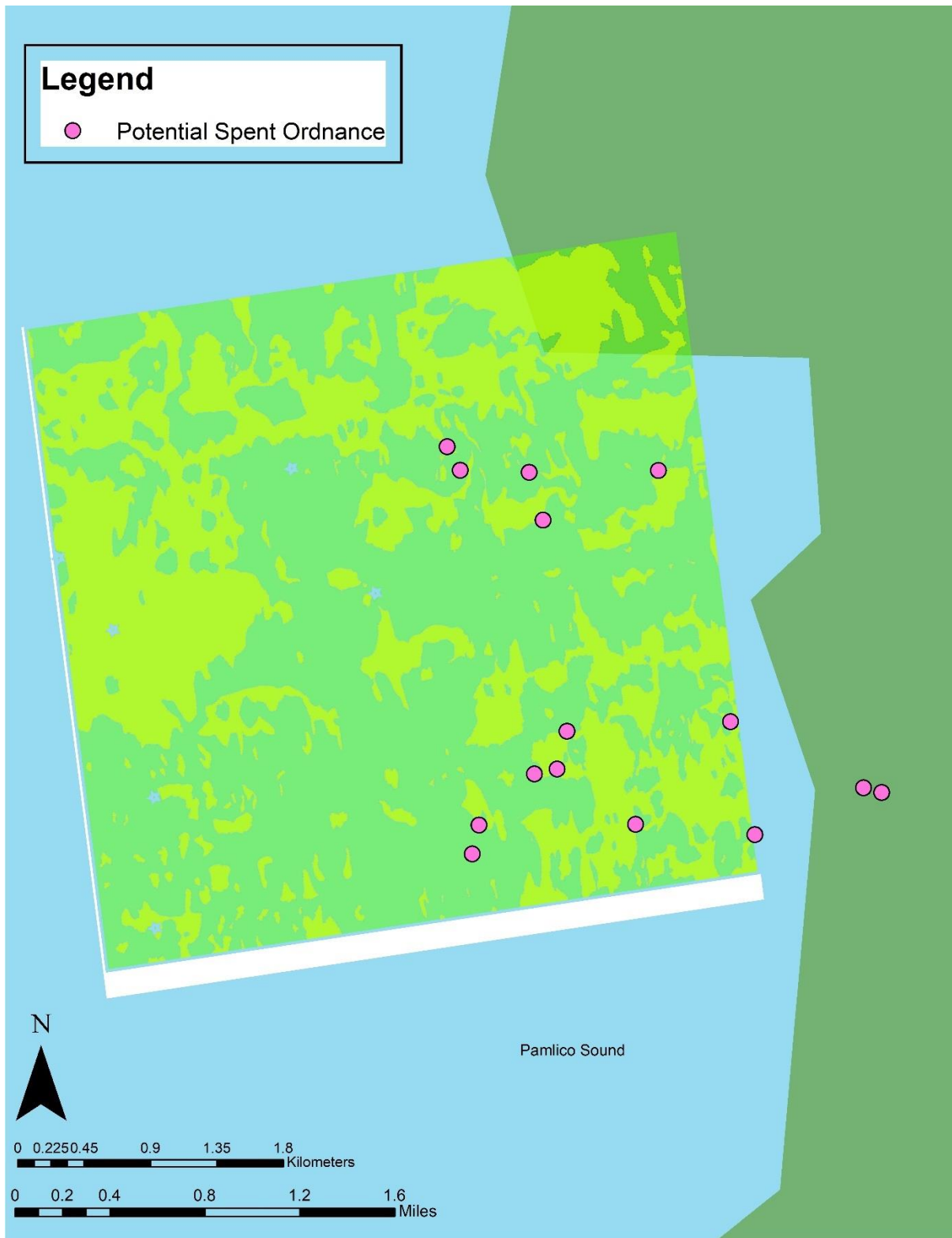
Figure 50. Map of Rodanthe depicting potential ordnance based off high ferrous and conductivity levels. Data was filtered according to a SQL statement. (By: Jim Kinsella).
