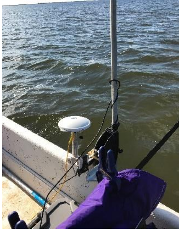
Figure 29. Pole mounted Tritech Sonar device with Trimble GPS unit (Photographed by Jim Kinsella).
