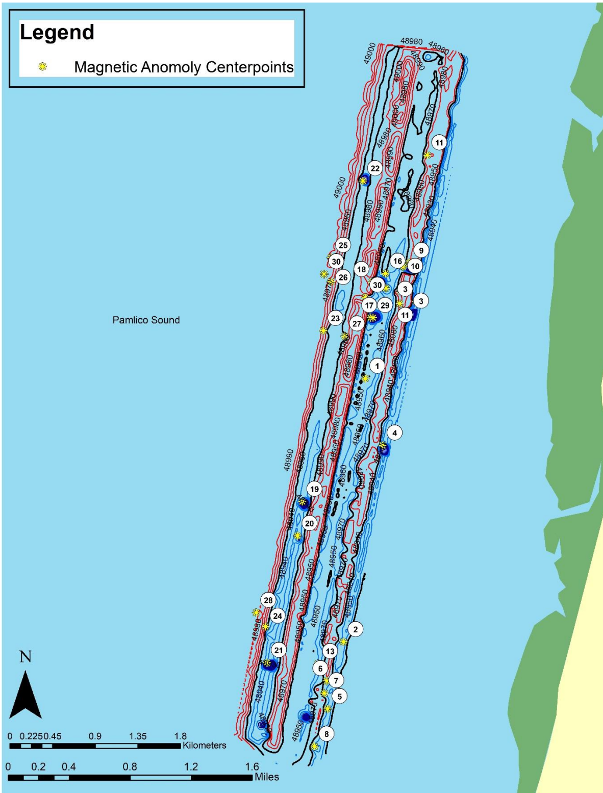
Figure 55. Magnetometer data from Hypack represented in the GIS model. Image includes 10m lane spacing with contour lines spaced at 10nT, as well as the epicenter for each magnetic anomaly. The epicenter of each anomaly is depicted by a yellow asterisk. (By Jim Kinsella)
