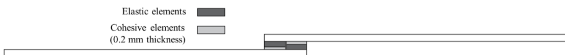
Fig. 10. Adhesive layer configuration used to model the behaviour of the SLJ with an adhesive thickness of 1.6 mm, with cohesive and plain strain elements being applied.
