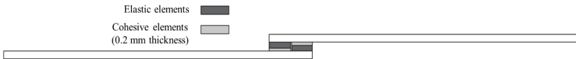
Fig. 8. Joint design used to model the behaviour of the SLJs with an adhesive thickness of 1.6 mm, with plain strain and cohesive elements being applied in the bonded region.
