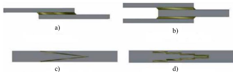
Figure 39 - Joint configurations: a) SLJ, b) DLJ, c) Double scarf joint, d) Double stepped-lap joint (adapted from [59])
