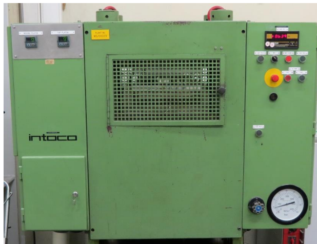
Figure 47 – Hot plate press used to cure the adhesive layer
