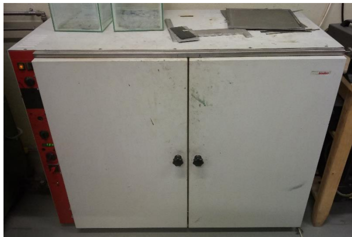
Figure 61 - Oven used to manufacture the front header joints
