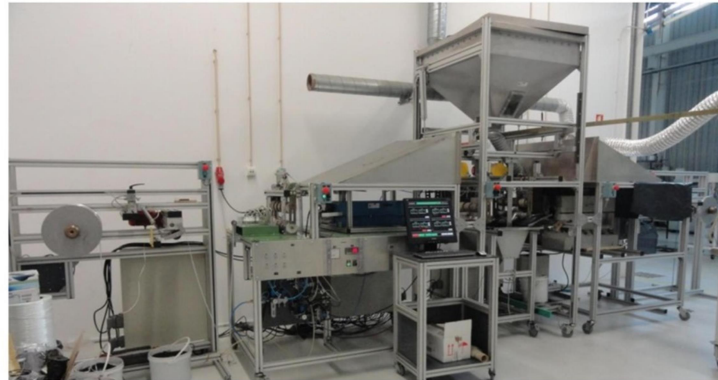
Figure 3. Prototype coating line equipment used to produce towpregs
