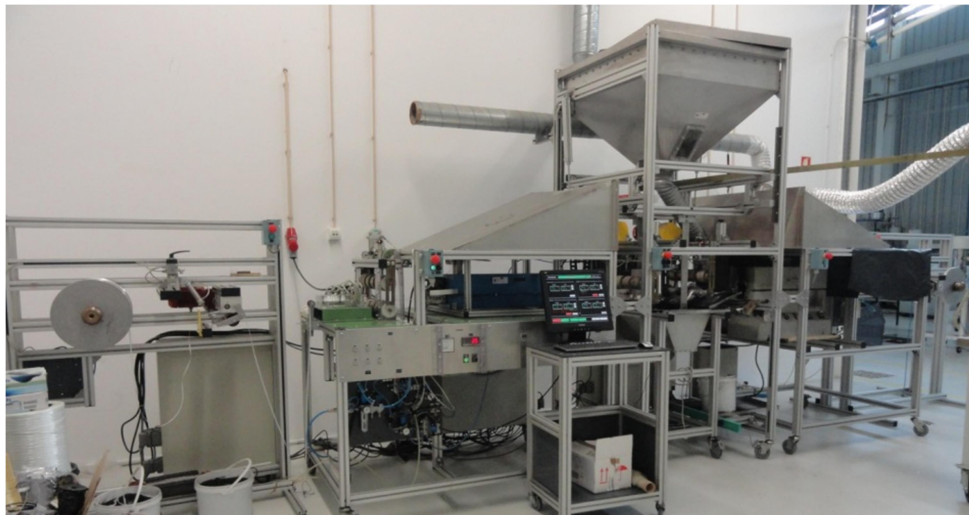
Figure 2. Powder coating line equipment used to produce towpregs
