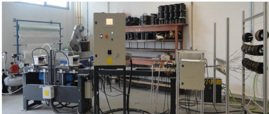
Figure 4. Developed prototype pultrusion line
