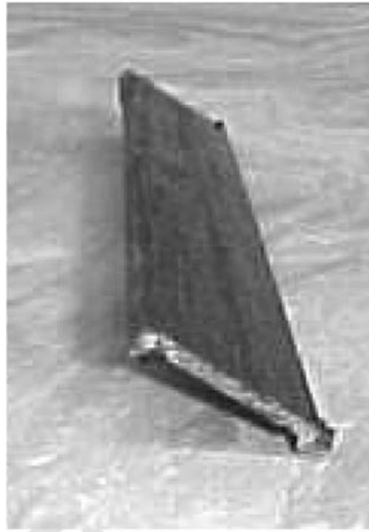
FIGURE 10. U-Shaped pultruded profile.
