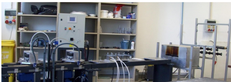
Figure 4. Overview of pultrusion equipment.
