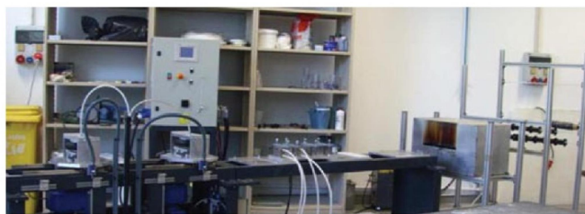
FIGURE 4. Overview of the proprietary pultrusion equipment.
