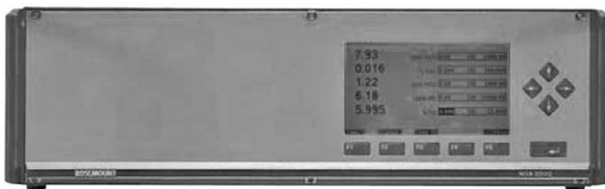
Figure 3. The NGA 2000 MLT Analyzer (Rosemount Analytical, Hasselroth Germany), used in papers 2 and 3, measures N_2O and CO_2 concentrations via absorption of infrared light.
