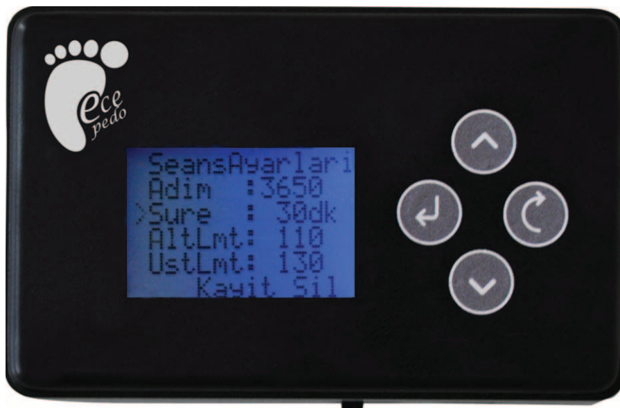
FIGURE 1. ECE PEDO: The session settings in the screen shows buttons of switching, recording and deleting to display lower limit, upper limit, number of steps, and walking time.
