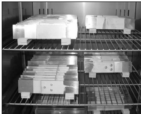
Fig. 3. The joints in climatic cabinet, at 50°C and 95 % Rh.
