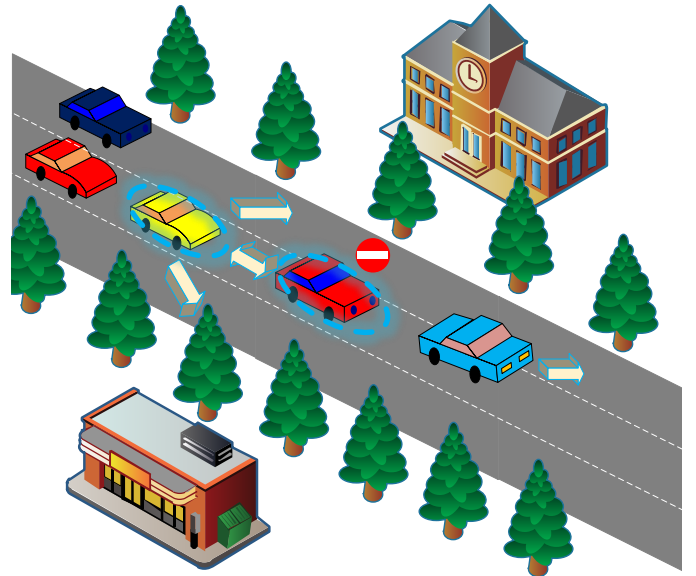
Fig. 2. Supplement of NLOS (no line of sight) traffic information for autonomous decision-making system
