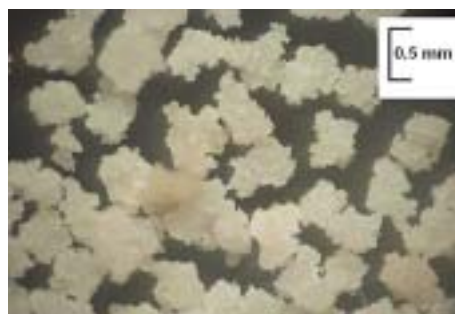
Fig. 2. Optical microscopic image of PVAm/DVB-I particles obtained in paraffin oil as continuous phase (after hydrolysis)
