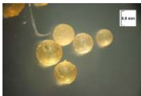
Fig. 4. Optical microscopic image of PVAm/DVB-II beads obtained in silicone oil as continuous phase (after hydrolysis)
