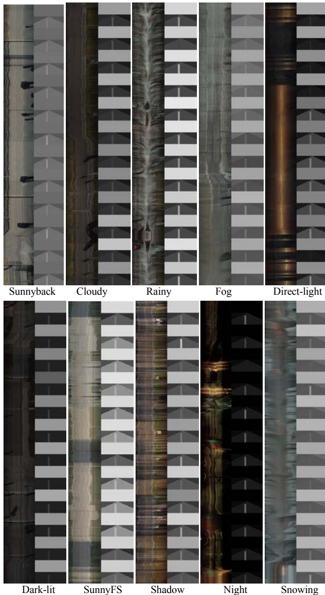
Figure 8 Comparison of road profile with approximated views on road and off-road for different weather clusters. Left of each figure is road profile and right column is a series of frames generated from sparse coding (linear combination of 17 basis). The sky is brighter than lower ground except night. The frame top is aligned with the frame position in road profile.
