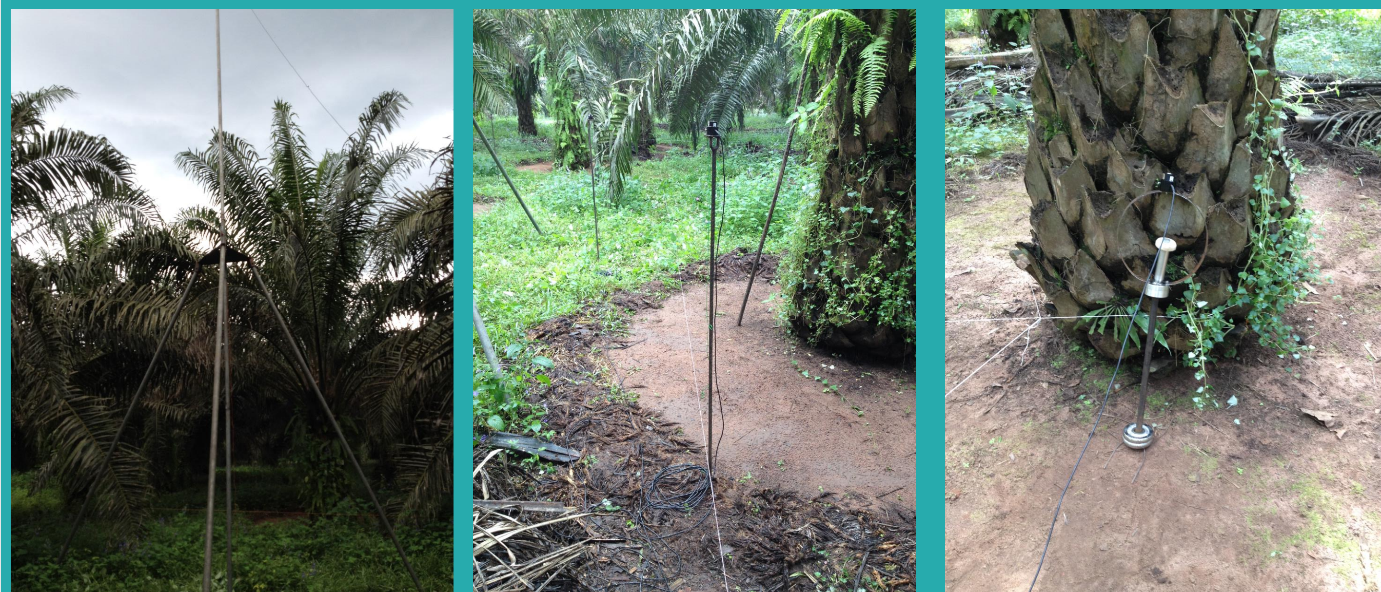
Figure 1 Left: device for measuring PAR above canopy. Middle: sensor measuring PAR below canopy for the fixed method. Right: quantum sensor on mobile levelling device for mobile sampling.
