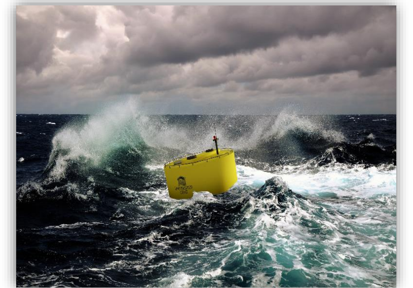
Fig. 2: Heaving WEC in extreme wave conditions.
