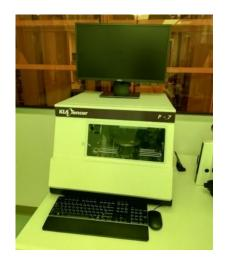
Figure C-12. KLA-Tencor P-7 Surface Profilometer.
