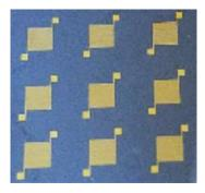
Figure 46. SOI wafer containing several membranes.
