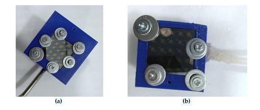
**Figure 54.** Burst pressure test setup with 3D printed test fixture involving (a) N<sub>2</sub> gas; (b) water.
