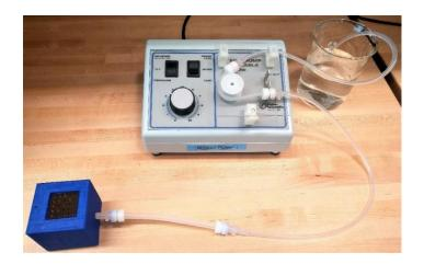
Figure 77. Setup for water flow testing.
