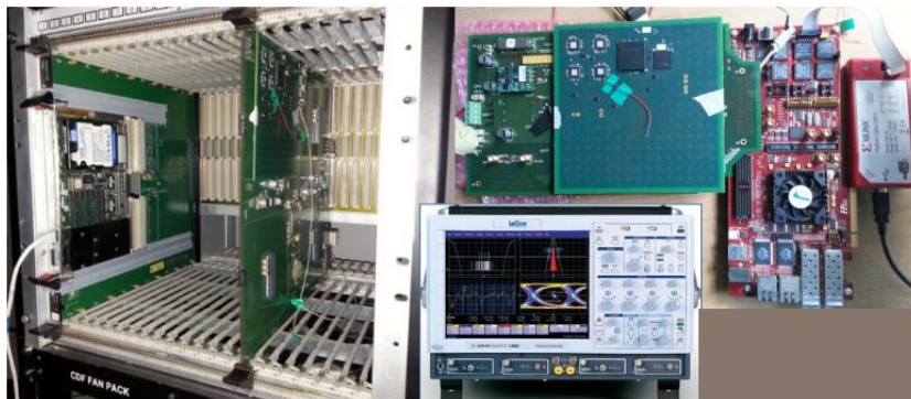
Figure 4: Test stands available in our lab. The left one is a VME crate while the right one is a stand-alone test for the LAMBSLP board.
